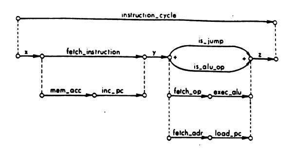
Figure 2-2: Illustration of the Timing Hierarchy
