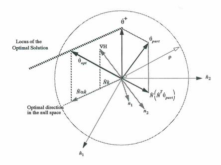
Figure 2: Velocity-based solution optimization using the reduced Jacobian approach
