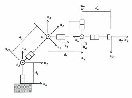
Figure 3: The AAI arm structure.
