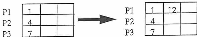
(g) Reduction: Task P1 gets the sum of three numbers, one from each of the three tasks, i.e., 1+4+7=12
