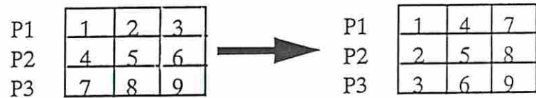
(f) Total Exchange: Every task sends a distinct message to each of the three tasks
