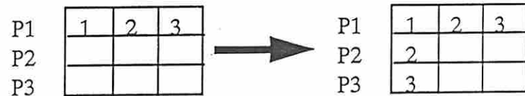
(d) Scatter: Task P1 sends a distinct message to each of the three tasks
