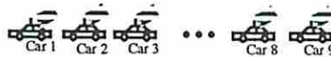
Fig. 4.2. Network A: Each and every of the 9 cars interferes and is interfered by all other cars.
