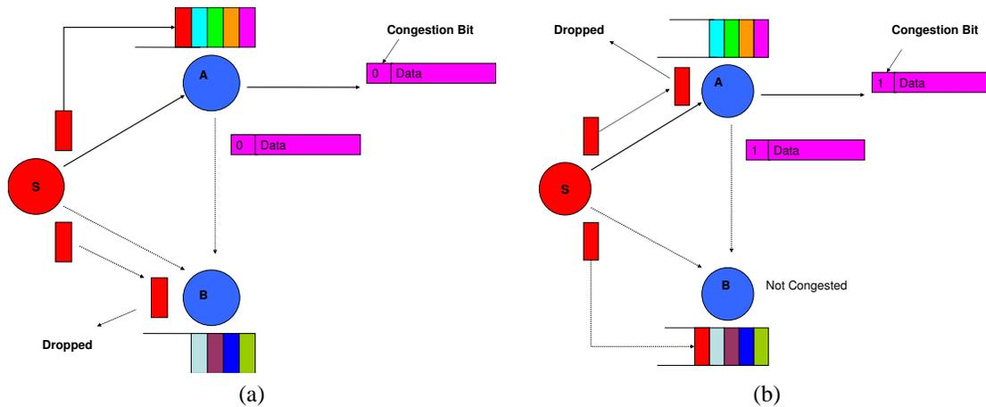
Fig. 1. (a) If  $A$  is not congested (congestion bit is reset),  $B$  drops the packet. (b) If  $A$  is congested (congestion bit is set),  $B$  stores the packet if it is not congested and  $A$  drops the packet.
