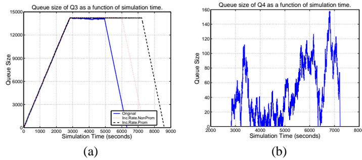
Fig. 5. Queue sizes of forwarding nodes 3 (a) and 4 (b) as a function of the simulation time for increased source data rates  $\{\lambda_0 = 10, \lambda_1 = 10, \lambda_2 = 4\}$  and constant queue sizes. The figures plot the *original* statistics (when the source data rate is not increased), *increased rate non promiscuous mode* statistics (when the wireless advantage is not used) and *increased rate promiscuous mode* statistics (when the wireless advantage is used).
