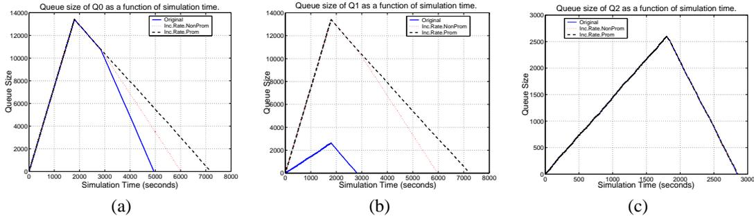
Fig. 4. Queue sizes of source nodes 0 (a) 1 (b) and 2 (c) as a function of the simulation time for increased source data rates  $\{\lambda_0 = 10, \lambda_1 = 10, \lambda_2 = 4\}$  and constant queue sizes. The figures plot the *original* statistics (when the source data rate is not increased), *increased rate non promiscuous mode* statistics (when the wireless advantage is not used) and *increased rate promiscuous mode* statistics (when the wireless advantage is used).
