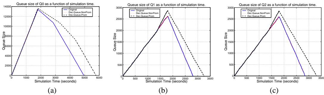
Fig. 6. Queue sizes of source nodes 0 (a) 1 (b) and 2 (c) as a function of the simulation time for reduced queue size at node 3 to 7000 packets from 14300 packets and when source data rates remain unchanged. The figures plot the *original* statistics (when the queue size is not reduced), *decreased queue size non promiscuous mode* statistics (when the wireless advantage is not used) and *decreased queue size promiscuous mode* statistics (when the wireless advantage is used).
