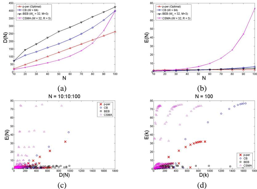
Fig. 12. Comparison of p-persistent slotted Aloha, slotted Aloha with constant back-off (CB), slotted Aloha with Binary exponential back-off (BEB) and slotted CSMA with constant window size.
