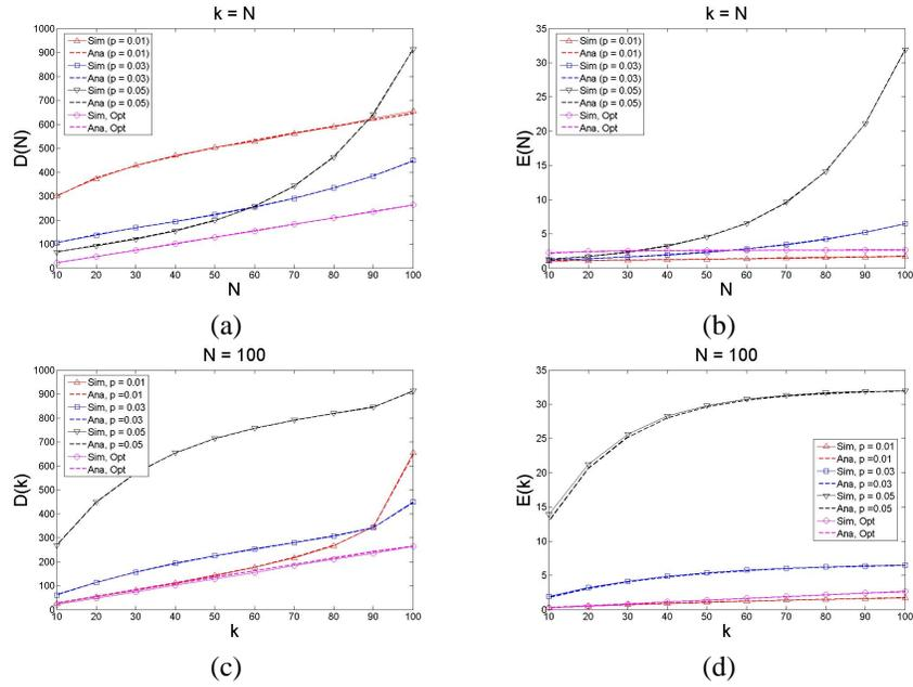
Fig. 7. Comparison of Analysis and Simulations for p-persistent Slotted Aloha.
