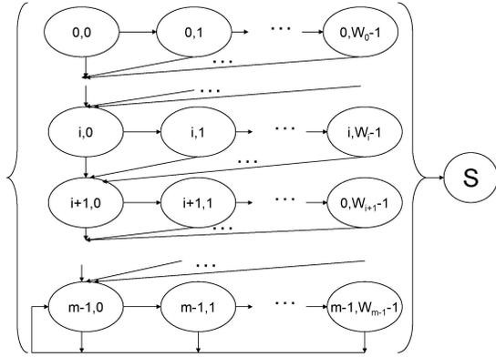
Fig. 3. Markov chain of states for a contending node using slotted Aloha with binary exponential back-off protocol.
