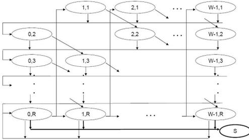
Fig. 4. Markov Chain for slotted CSMA with constant back-off.
