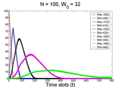
Fig. 9. Comparison of Analysis and Simulations for slotted Aloha with Binary Exponential Back-off.
