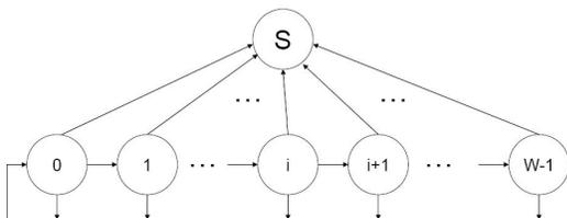
Fig. 2. Markov chain of states for a contending node using slotted Aloha with constant back-off protocol.
