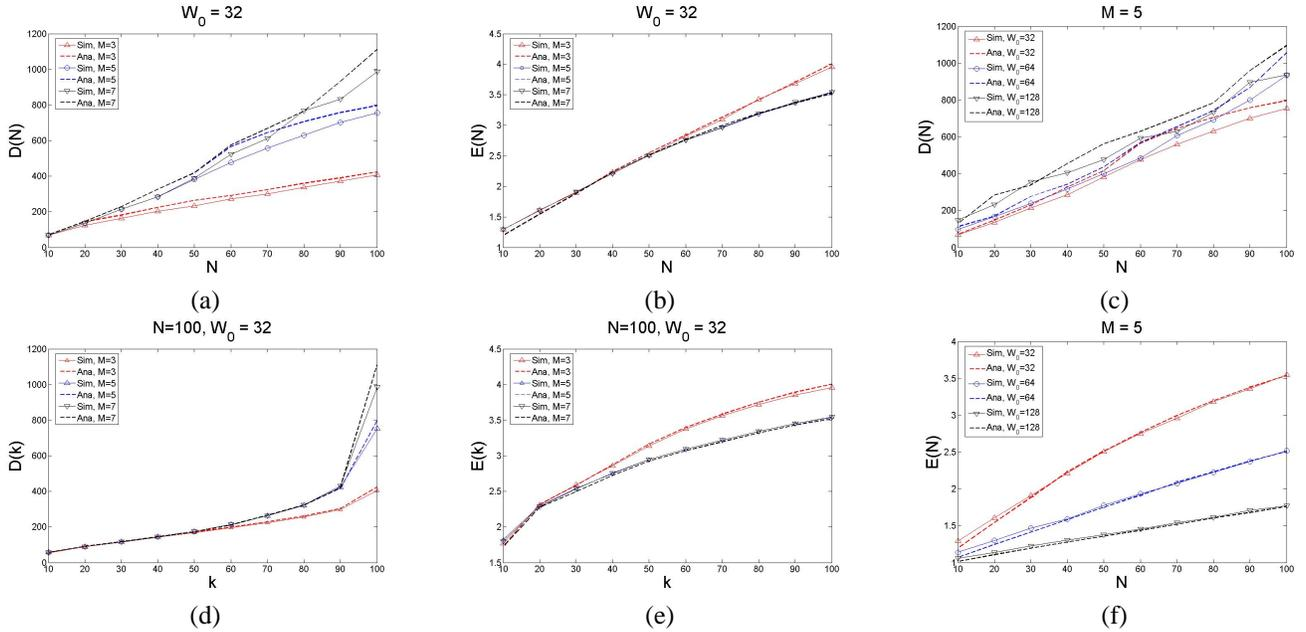
Fig. 10. Comparison of Analysis and Simulations for slotted Aloha with Binary Exponential Back-off.
