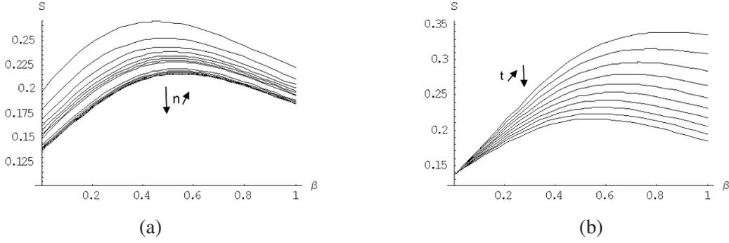
Fig. 3. Throughput of PDT-ALOHA vs.  $\beta$ ; (a) when  $t = 1$  and  $n$  is variable, (b) when  $n = 100$  and  $t$  is variable.
