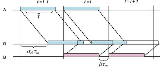
Fig. 1. Time diagram of packet transmission;  $A$  and  $B$  are transmitters and  $R$  is the receiver.  $B$  locates closer to the receiver than  $A$ .
