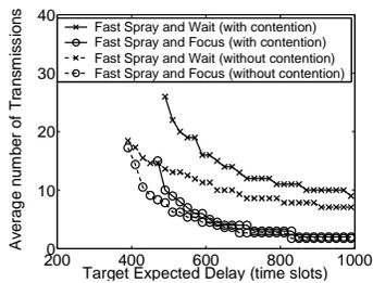
Fig. 7. Comparison of fast spray and wait and fast spray and focus. Average number of transmissions required to deliver the packet to the destination vs target expected delay. Network parameters:  $N = 500 \times 500$  square units,  $M = 40$ ,  $K = 20$ ,  $\Theta = 5$ ,  $s_{BW} = 1$  packet/time slot,  $p_l = 0.8$ ,  $p_r = 0.15$ ,  $r = 4$ .
