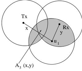
Fig. 2. Tx and Rx denote the transmitter and the receiver. Node  $u_1$  is a node within the scheduling area and at a distance  $x$  from the transmitter and at a distance  $y$  from the receiver. The shaded area represents  $A_3(x, y)$ .
