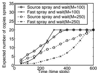
Fig. 6. Comparison of fast spray and wait and source spray and wait: Expected number of copies spread vs time elapsed since the packet was generated. Network parameters:  $N = 100 \times 100$  square units,  $K = 5$ ,  $\Theta = 5$ ,  $s_{BW} = 1$  packet/time slot,  $L = 20$ . Expected maximum cluster size (metric to measure connectivity) for these network parameters is equal to 4.6% for  $M = 100$  and 5.2% for  $M = 250$ .
