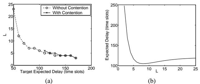
Fig. 5. (a) Minimum value of  $L$  which achieves the target expected delay for source spray and wait. (b)  $L$  against expected delay (with contention). Network parameters:  $N = 100 \times 100$ ,  $K = 8$ ,  $M = 150$ ,  $\Theta = 5$ ,  $E[S] = 70$ ,  $T_{stop} = 0$ ,  $\bar{v} = 1$ ,  $s_{BW} = 1$ .
