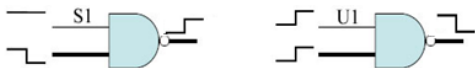
Figure 4: Conditions for robust path delay testing for an on-path NAND gate. The thick and thin lines denote on-path and off-path lines, respectively.
