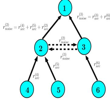
Fig. 1. A 6 node topology: An illustrative example of the receiver capacity model
