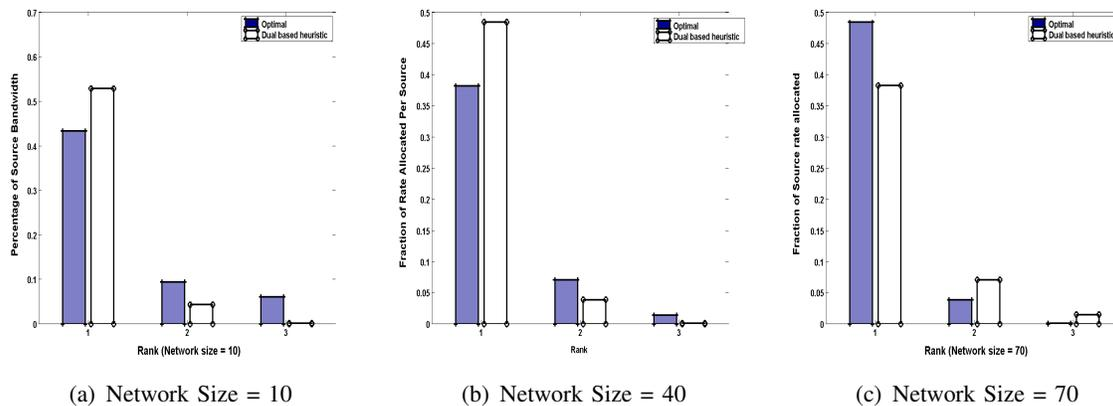
Fig. 8. The distributions of the percentage of the total rate that was allocated to a source belonging to a particular rank for different network sizes. The skewed distributions highlight that a few sources are allocated a large percentage of the available bandwidth in order to maximize the utilization.
