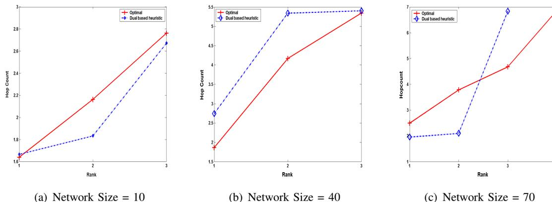
Fig. 10. The dependence of rank on hop count. The largest ranks are much farther away from the root as compared to the hop count of the smaller ranks.
