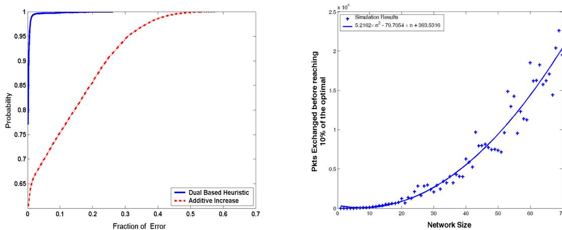
(a) CDF of the error observed between the optimal throughput achievable and the throughput achieved using dual based algorithm and the additive increase algorithm. (b) Performance of the algorithm in terms of the number of packets exchanged before achieving 10% of the optimal.
