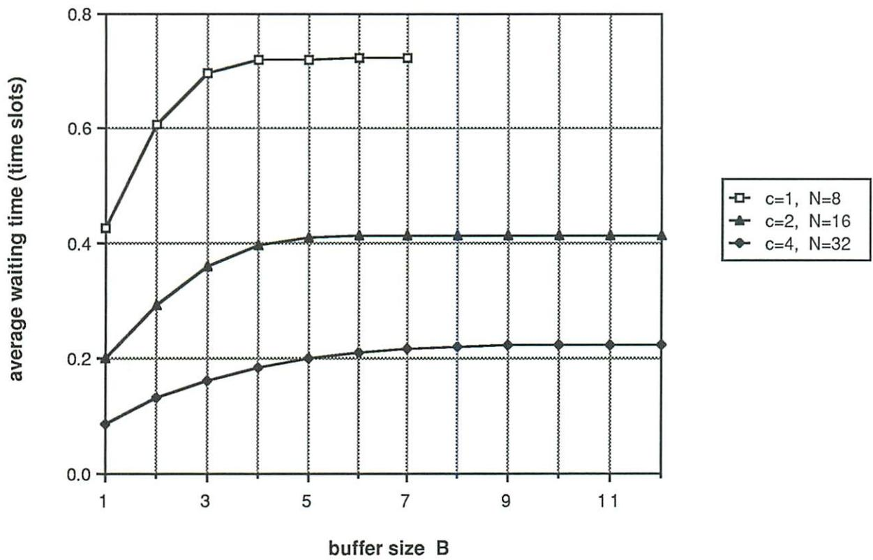
Fig. 5: The average waiting time as a function of B for F=10 and various c.
