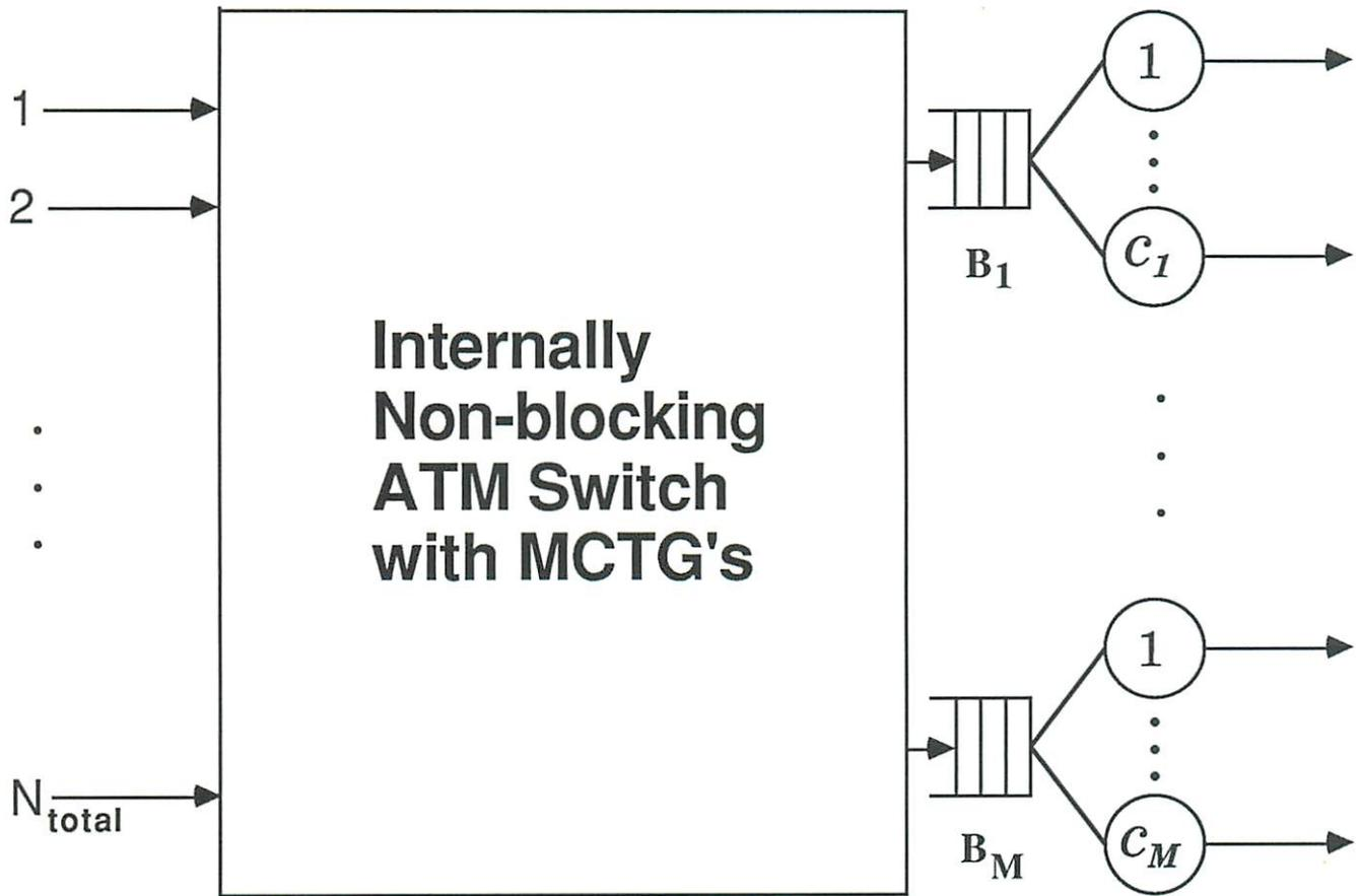
Fig. 1: The system model of an internally nonblocking ATM switch with multichannel transmission groups (MCTG).
