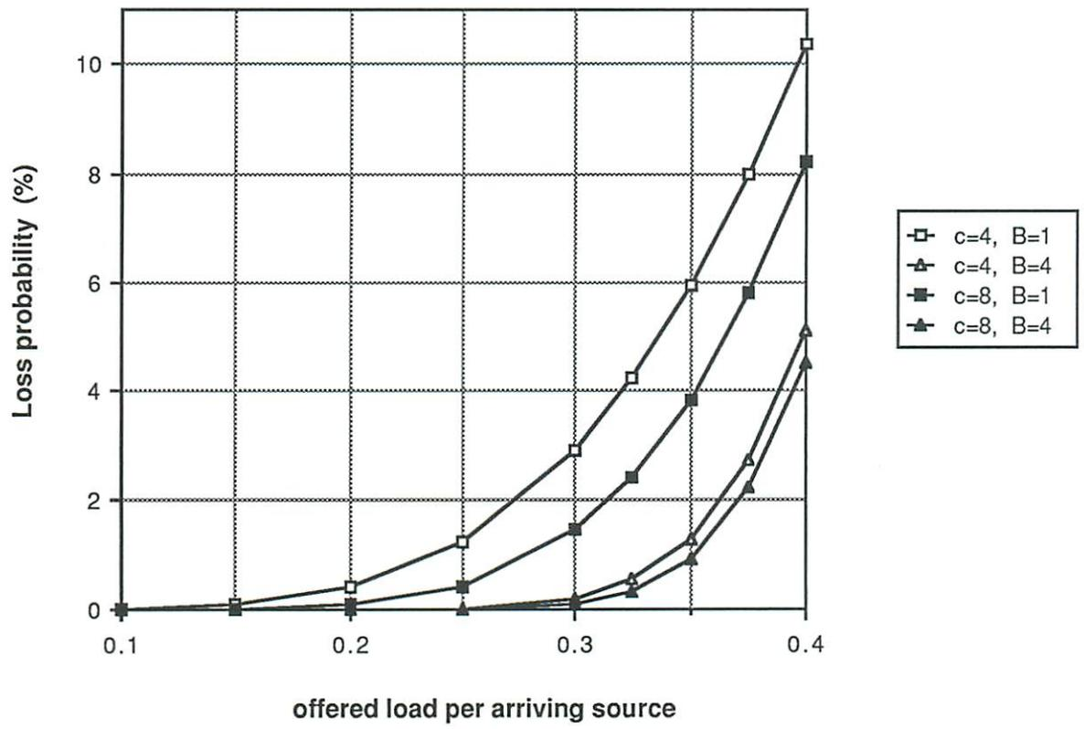
Fig. 4: The loss probability for  $c=4, N=10$  and  $c=8, N=20$ , and various  $B$ .
