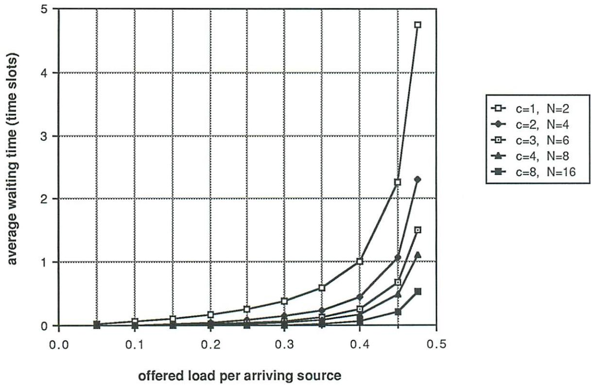
Fig. 2: The average waiting time for various cases of  $N=2c$  assuming infinite buffer.
