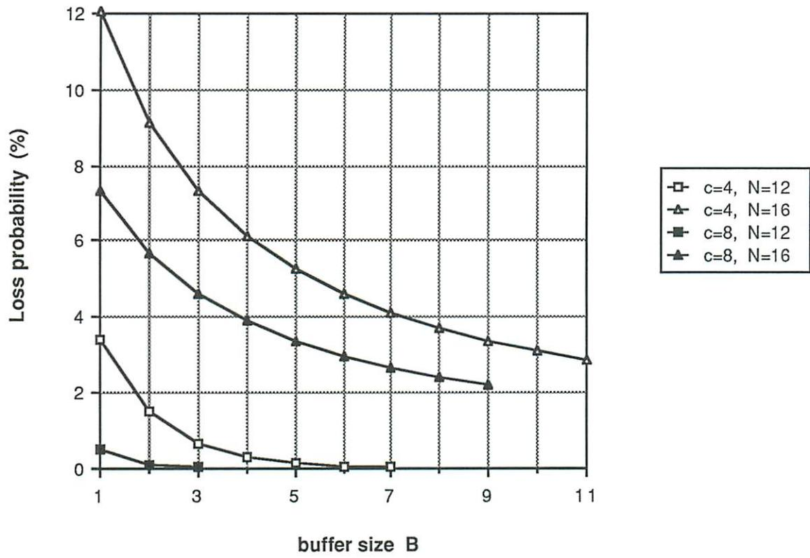
Fig. 3: The loss probability as a function of B and N, for  $c=4$ ,  $p=0.25$  and  $c=8$ ,  $p=0.5$ .
