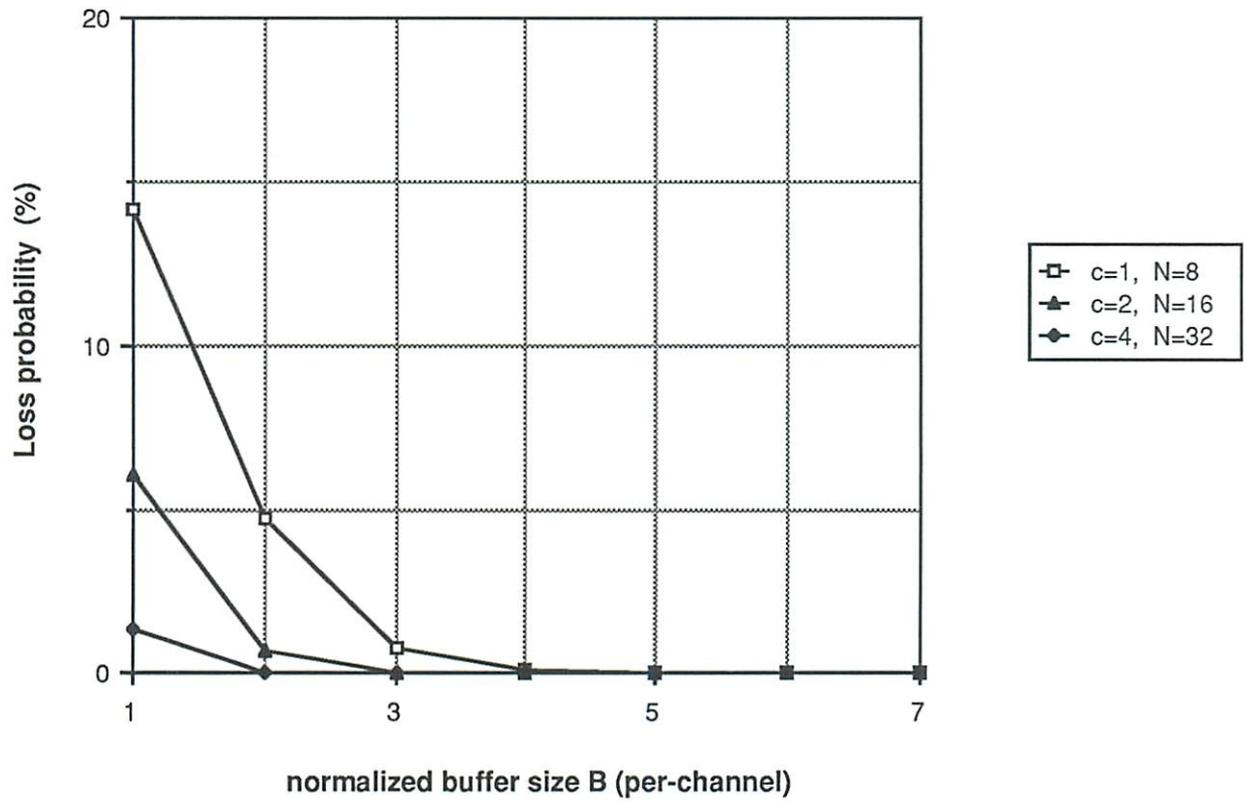
Fig. 6: The loss probability as a function of normalized B for  $F=10$  and various  $c$ .
