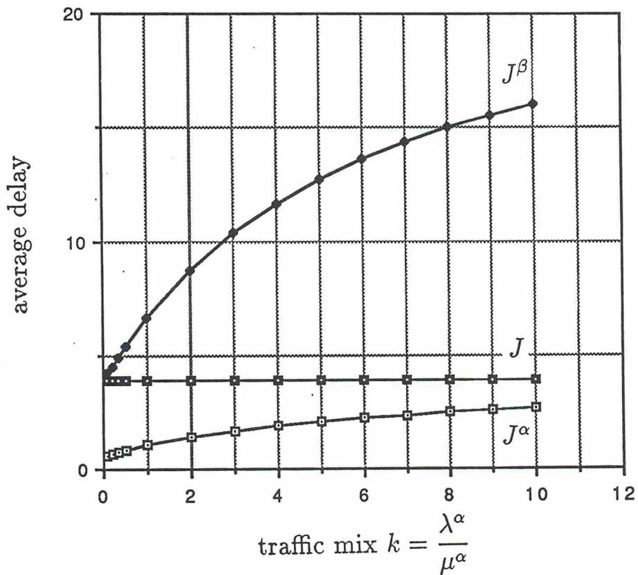
Fig. 2 Stackelberg equilibrium average delay  $J^\alpha$ ,  $J^\beta$  and  $J$  versus different mix of the high and low priority arrival rates  $\frac{\lambda^\alpha}{\lambda^\beta}$ , for  $C_1 = 2, C_2 = 1, \lambda^\alpha + \lambda^\beta = 2.5$ , and  $\mu^\alpha = \mu^\beta = 1$ .
