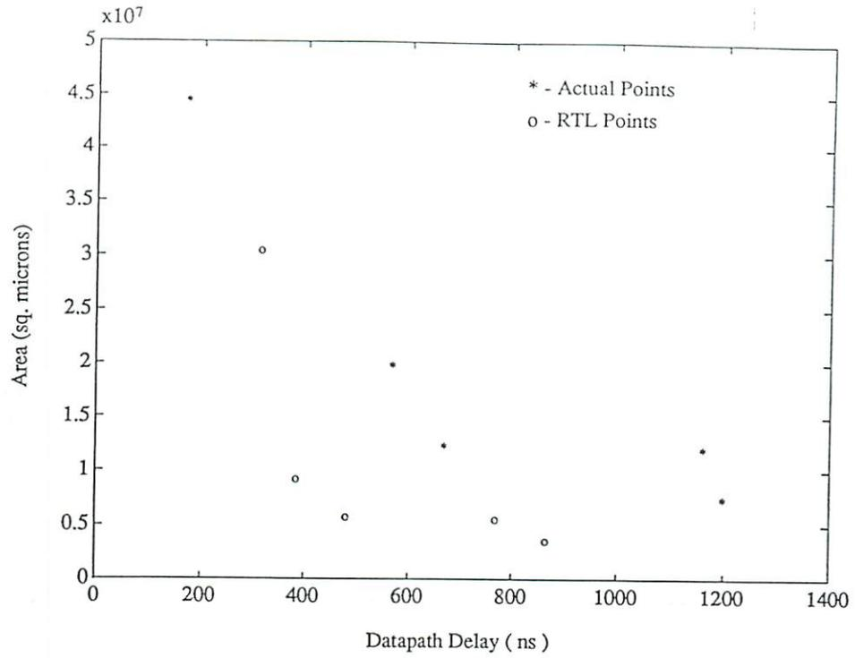
Figure 4: Cost-performance tradeoff curve for a 16-bit Non-Pipelined AR Filter Datapath Element
