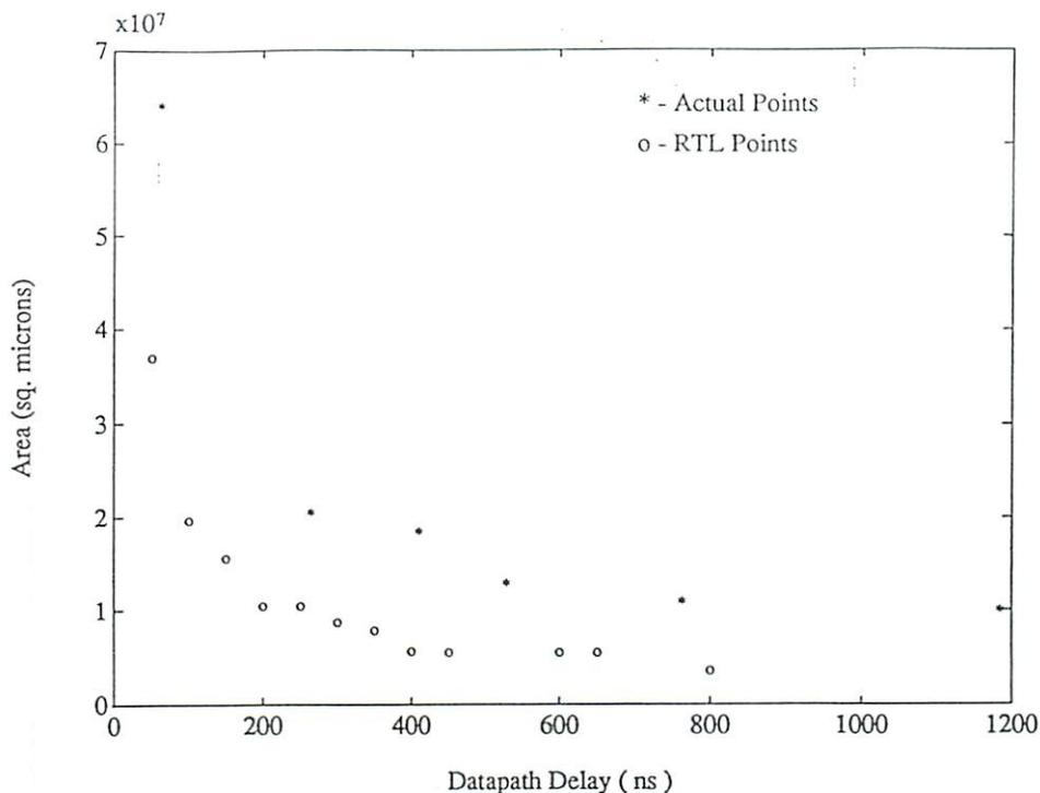
Figure 6: Overall Cost-performance tradeoff curve for a 16-bit Pipelined AR Filter Datapath
