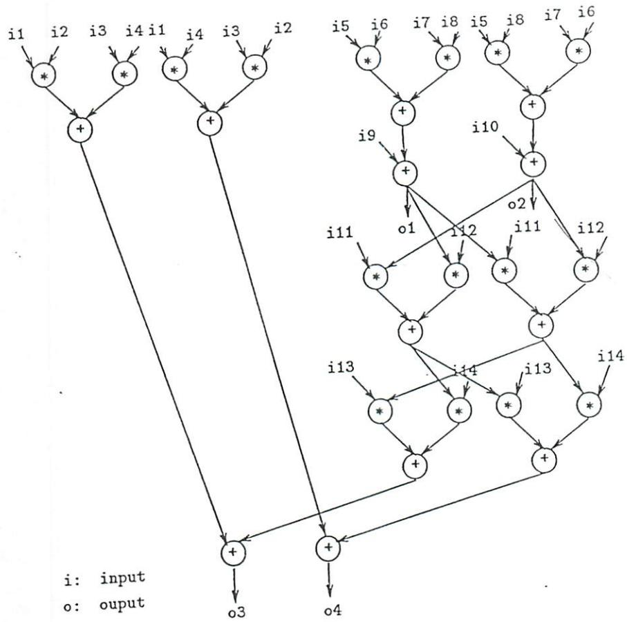
Figure 1: The AR Filter Dataflow Graph
