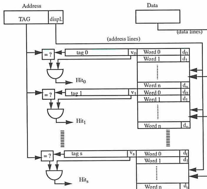
Figure 7: Block diagram of an ISB
