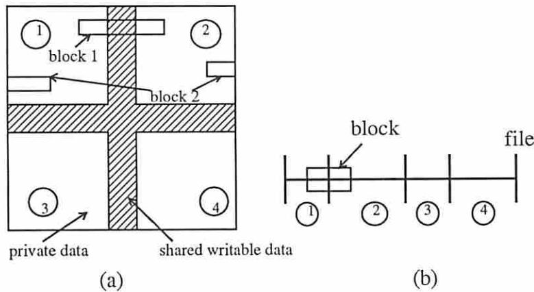
Figure 2: Illustration of false sharing in the S.O.R. (a) and Quicksort (b) algorithms
