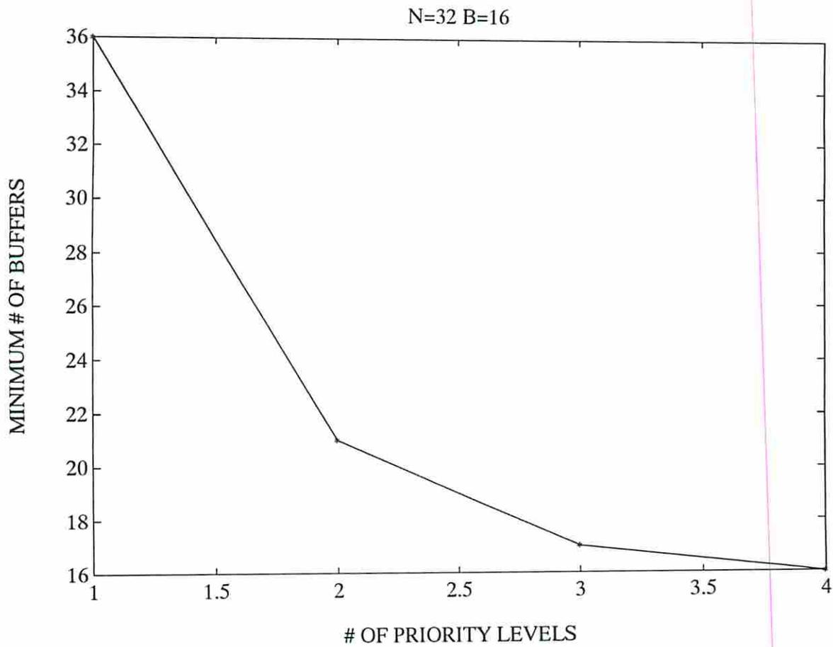
**Figure 3: buffer requirement to carry table 3 traffic scenario**
