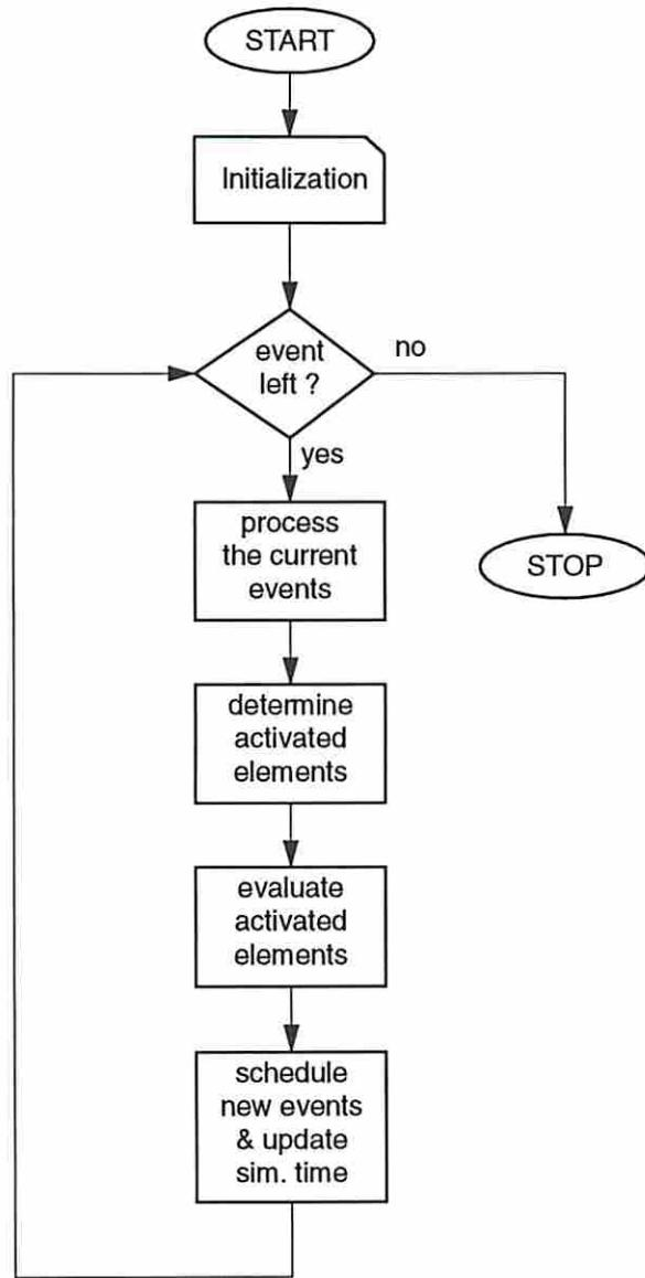
Figure 6: Typical flow of event-driven simulation
