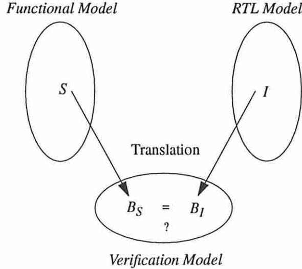
Figure 1: The verification model and its relationships with the functional and RTL models.
