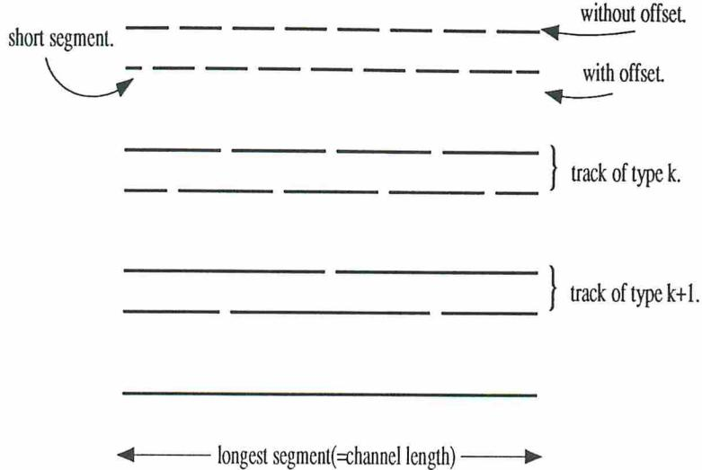
Figure 1: The FPGA Routing Channel
