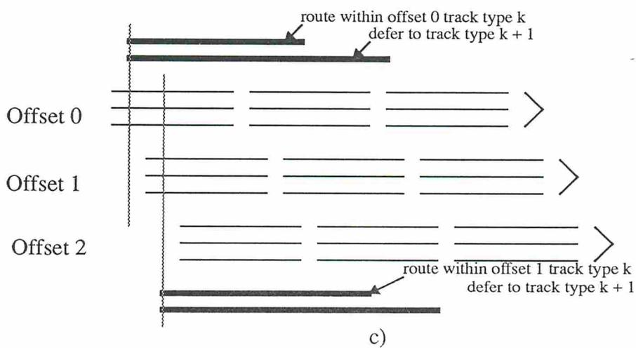
Figure 2: The staggered non-uniform segmentation model (shown for tracks of type  $k$ )
