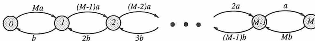
Fig. 2. Model for video sources with  $M+1$  levels of cell arrival rate.
