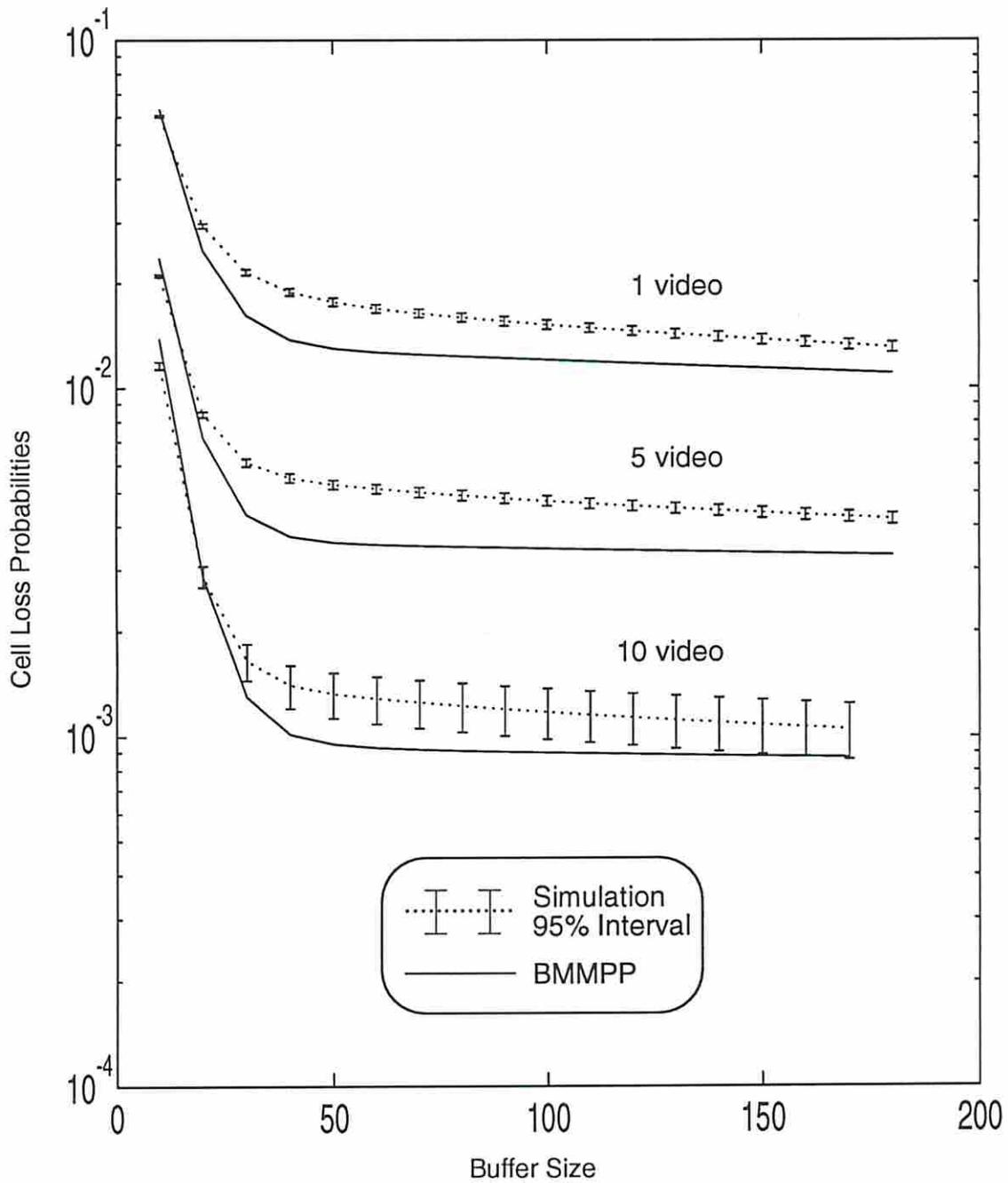
**Fig. 11** Cell loss probabilities for a system load of 0.8 and 100 voice calls and 100 data calls with different number of video calls.
