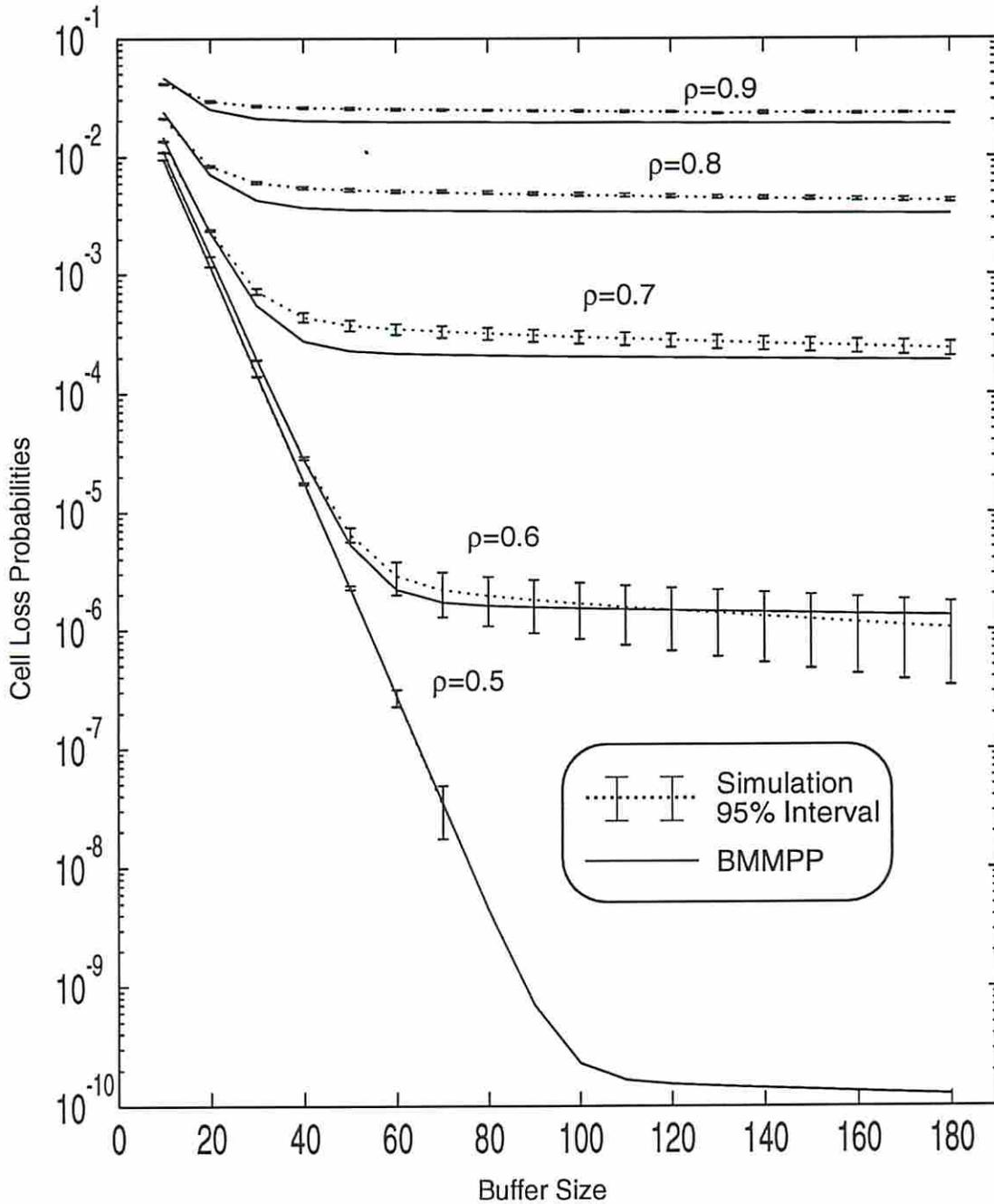
**Fig. 10** Cell loss probabilities for 5 video calls, 100 voice calls and 100 data call with different system loads.
