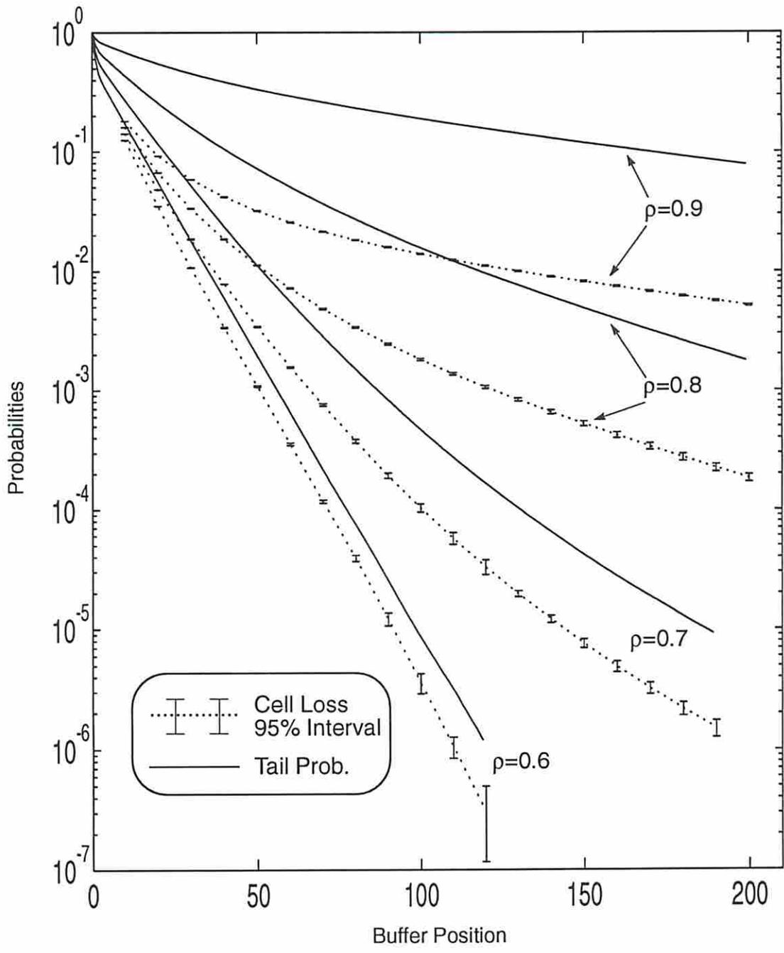
**Fig. 8** Tail probabilities versus loss probabilities for 20 voice calls and 50 data calls (simulation results).
