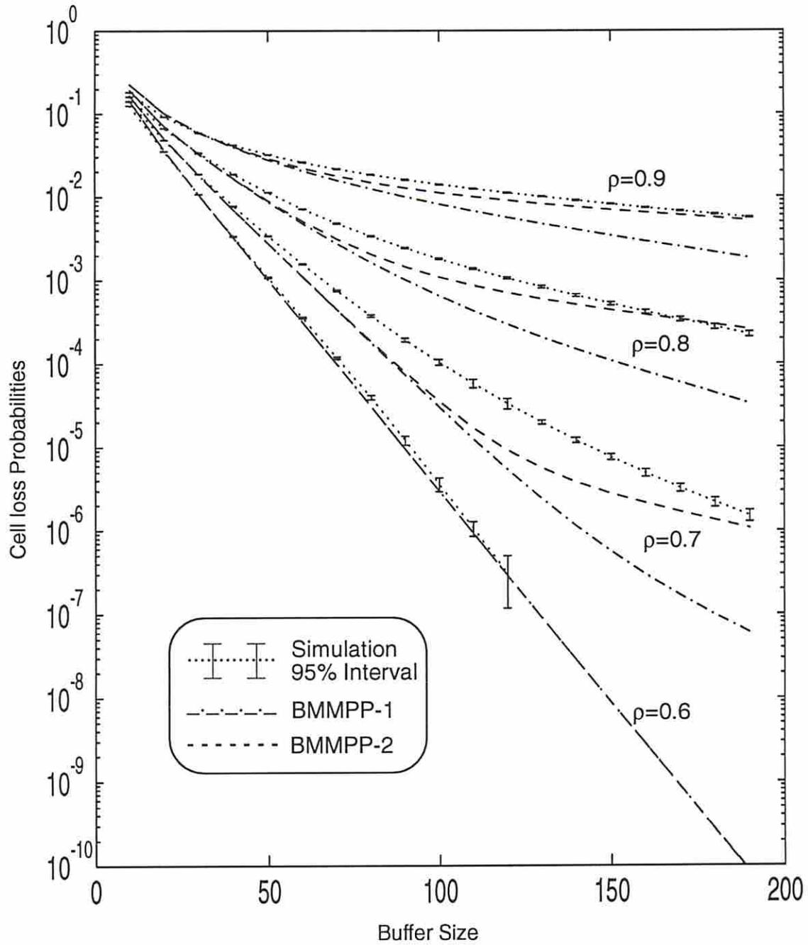
**Fig. 7** Cell loss probabilities for 20 voice calls and 50 data calls with different system loads.
