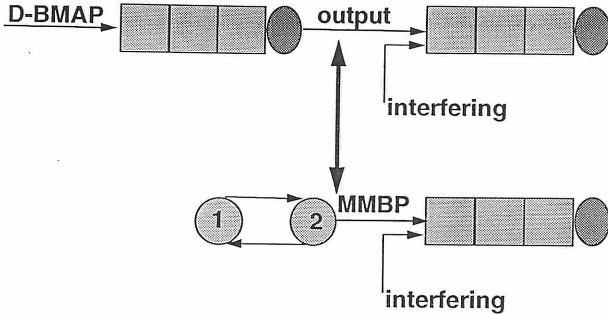
Figure 2: Scheme of the first set of experiments - the output process of the first queue was substituted by a two-state MMBP
