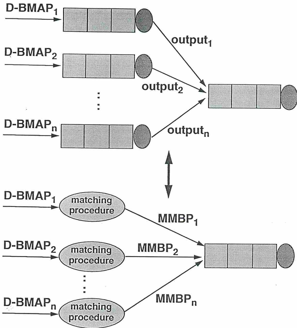
Figure 8: Scheme for the second set of experiments - the output of each queue was substituted by a two-sate MMBP
