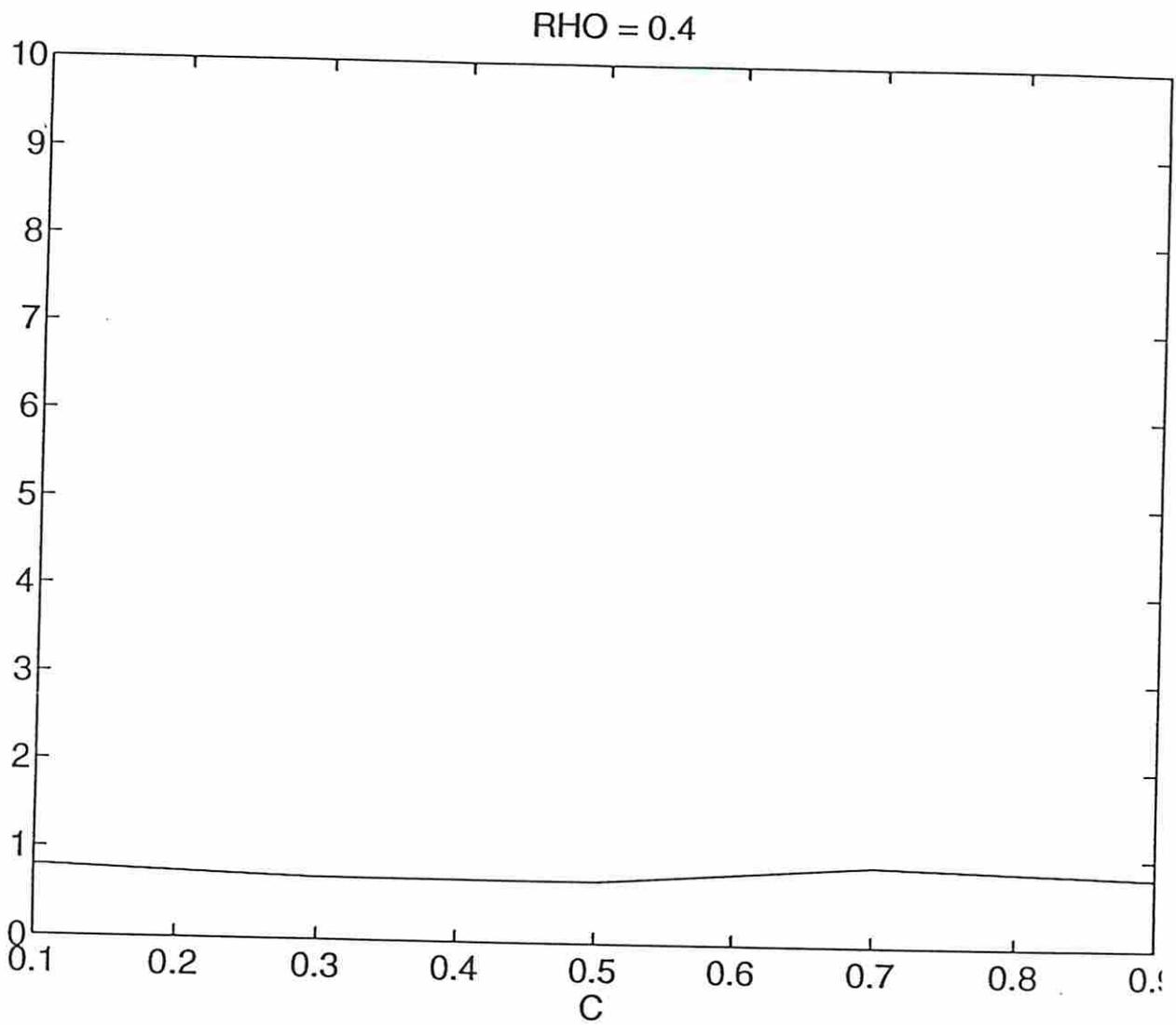
Figure 3: Percentual error of the delay estimation as a function of  $c$  (system load = 0.4)
