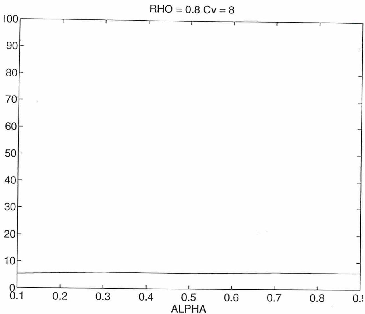
Figure 6: Percentual error of the delay estimation as a function of  $\alpha(\rho = 0.8, C_v = 8)$
