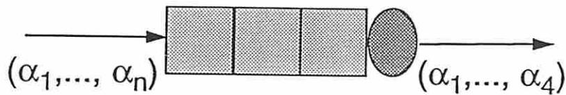
Figure 1: In product form networks the flow is characterized by the mean of a Poisson process. In queueing networks with renewal flow by the mean and the variance of the renewal process. In queueing networks with Markov modulated flow, the number of parameters depends on the size of the underlying Markov Chain. If the MC is a two state, we need four parameters.
