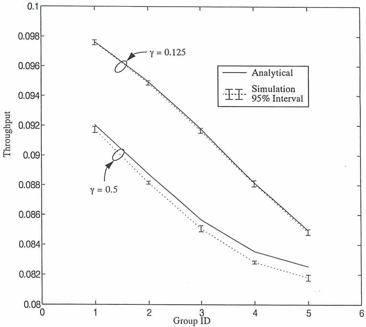
Fig. 2. Throughput for a 5-group system with  $\sigma = 0.02$ ,  $q = 0.1$ ,  $\delta = 1.0$ , and  $R = 4$ . Note that as  $\gamma$  decreases, throughput increases.
