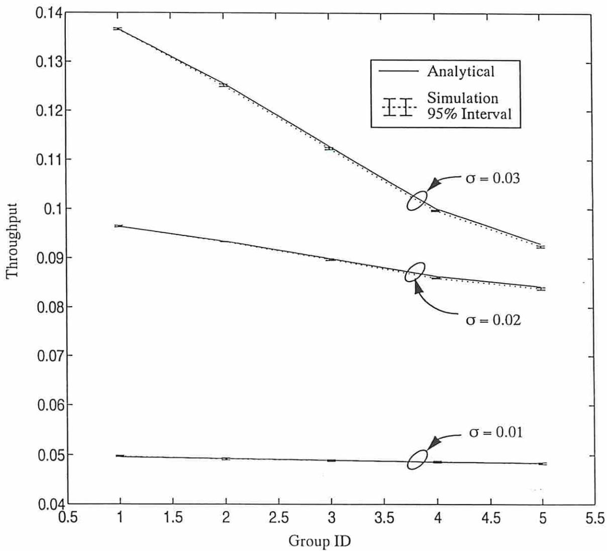
Fig. 6. Unbalanced throughput for a 5-group system with  $q = 0.1$ ,  $\gamma = 0.25$ ,  $\delta = 1.0$ , and  $R = 4$  for all groups.
