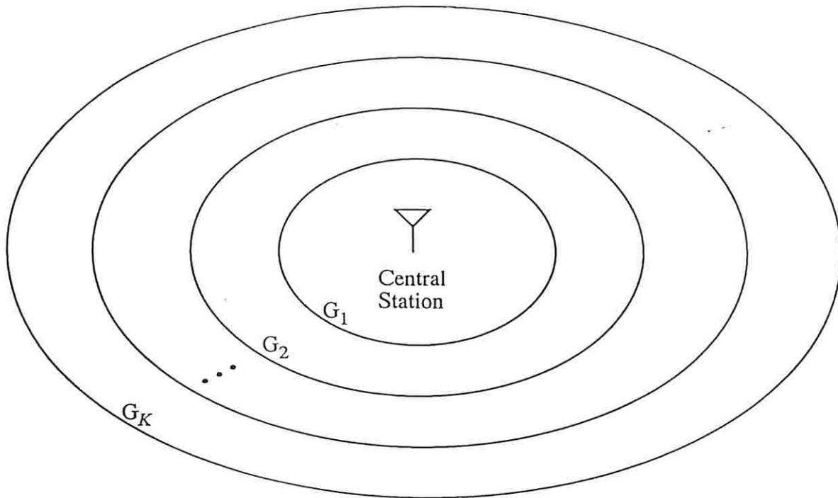
Fig. 1. The topology of a  $K$ -group slotted ALOHA system. All groups use the same transmission power. But due to the near-far effect, the received power at the central station is different.
