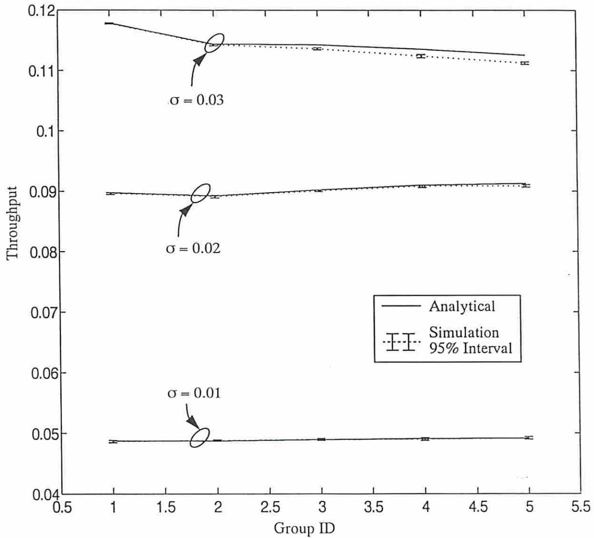
Fig. 7. Balanced throughput for a 5-group system with different retransmission probabilities for each group. Specifically,  $\gamma = 0.25$ ,  $\delta = 1.0$ , and  $R = 4$  for all groups;  $q_1 = 0.03$ ,  $q_2 = 0.055$ ,  $q_3 = 0.1$ ,  $q_4 = 0.16$ , and  $q_5 = 0.2$  for groups 1 through 5, respectively.
