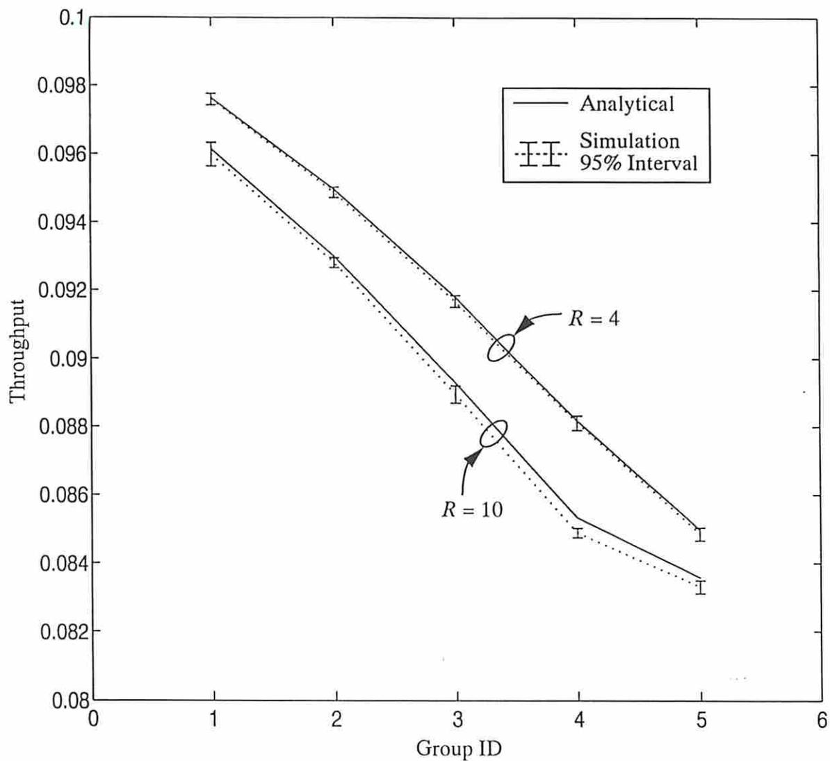
Fig. 3. Throughput for a 5-group system with  $\sigma = 0.02$ ,  $q = 0.1$ ,  $\gamma = 0.125$ , and  $\delta = 1.0$ . Note that as  $R$  decreases throughput increases.
