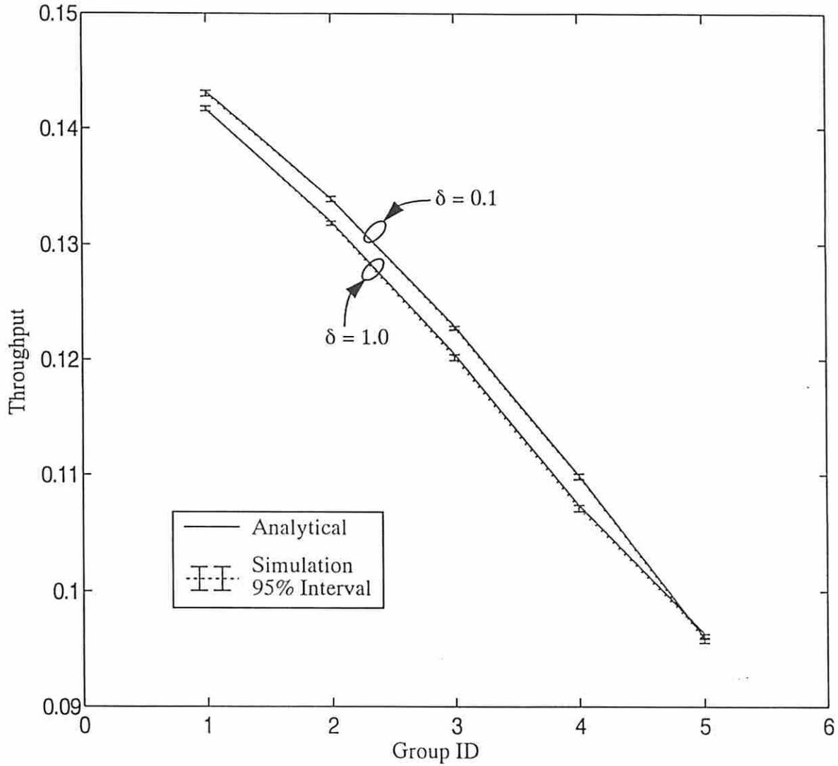
Fig. 5. In the cases where the near-far effect is significant (e.g.,  $\gamma = 0.125$  and  $R = 4$  in the example), throughput decreases as  $\delta$  increases. ( $\sigma = 0.03$  and  $q = 0.1$  for all groups.)
