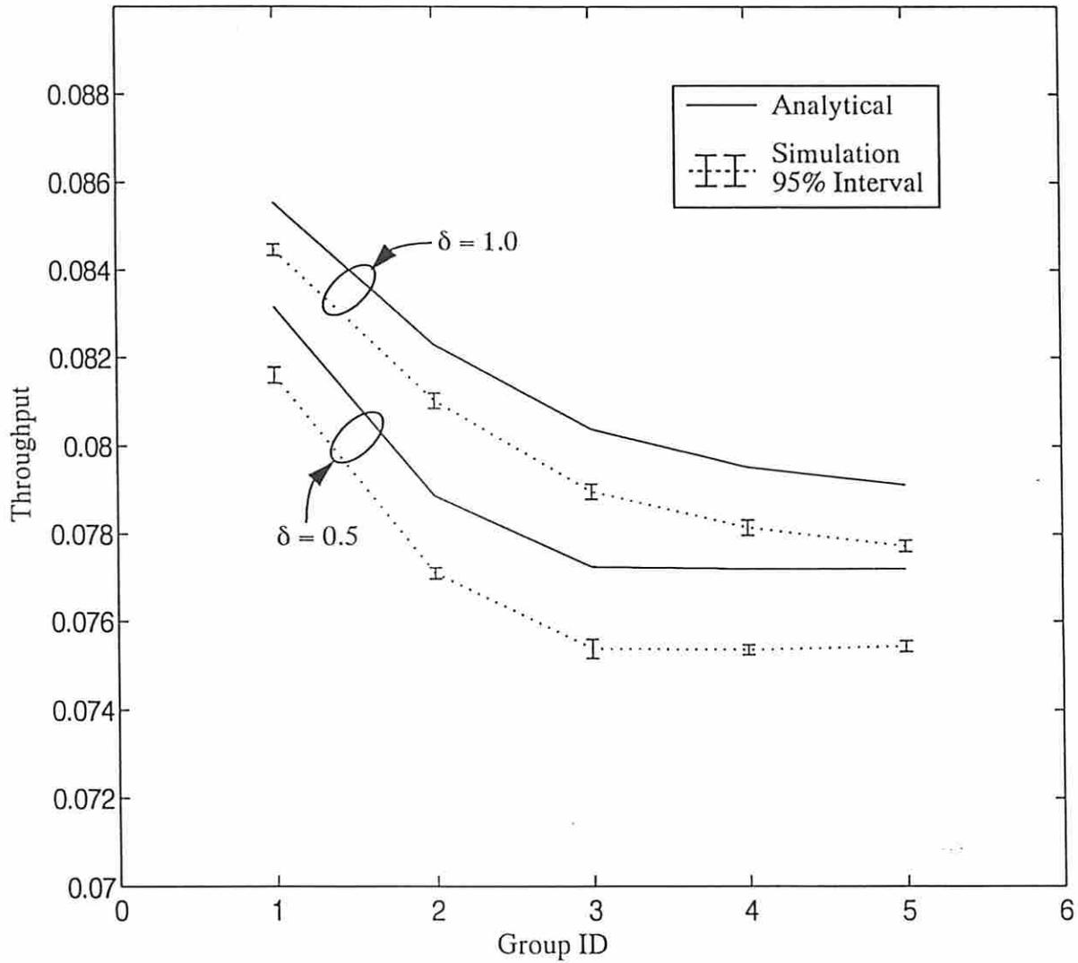
Fig. 4. Throughput for a 5-group system with different fading parameters ( $\delta$ ). In the cases where the near-far effect is not significant (e.g.,  $\gamma = 0.5$ ,  $R = 10$  in the example), throughput increases as  $\delta$  increases. (For other parameters,  $\sigma = 0.02$  and  $q = 0.1$  for all groups.)
