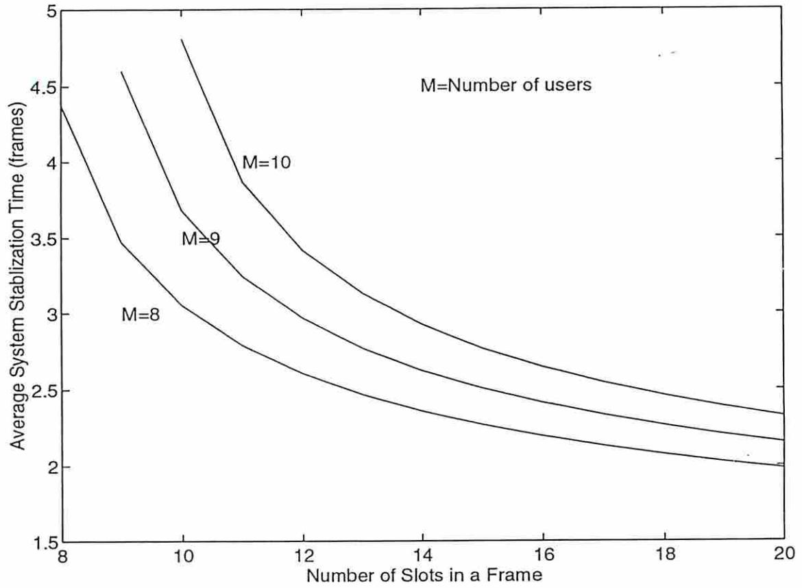
Fig. 5. The average system stabilization time as a function of  $M$  (number of users) and  $N$  (number of slots in a frame) for network A in the worst case.
