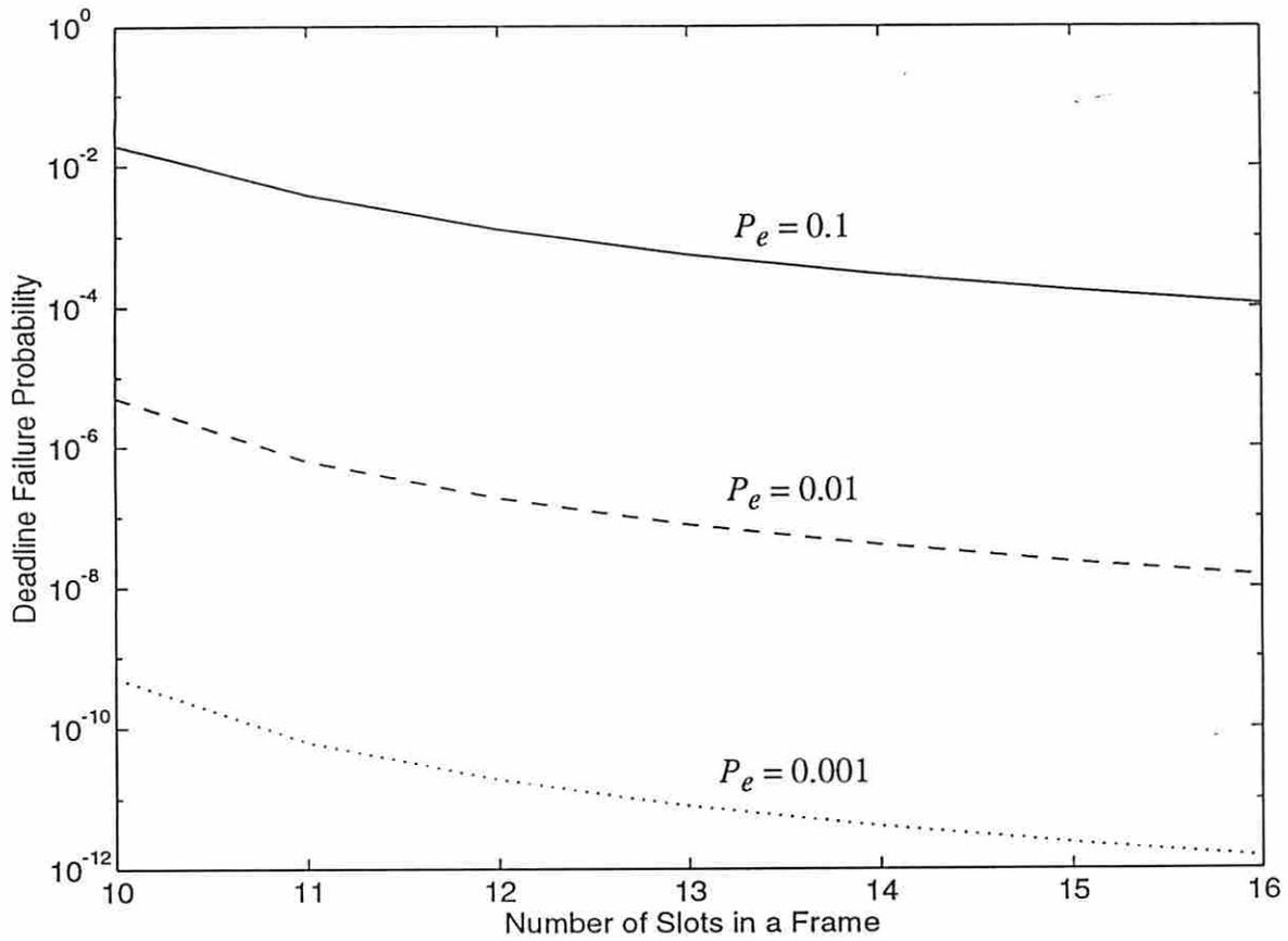
Fig. 10. The deadline failure probability as a function of the number of slots in a frame and the packet error probability ( $P_e$ ) for network B in the steady state. The deadline period is assumed to be 4 frames.
