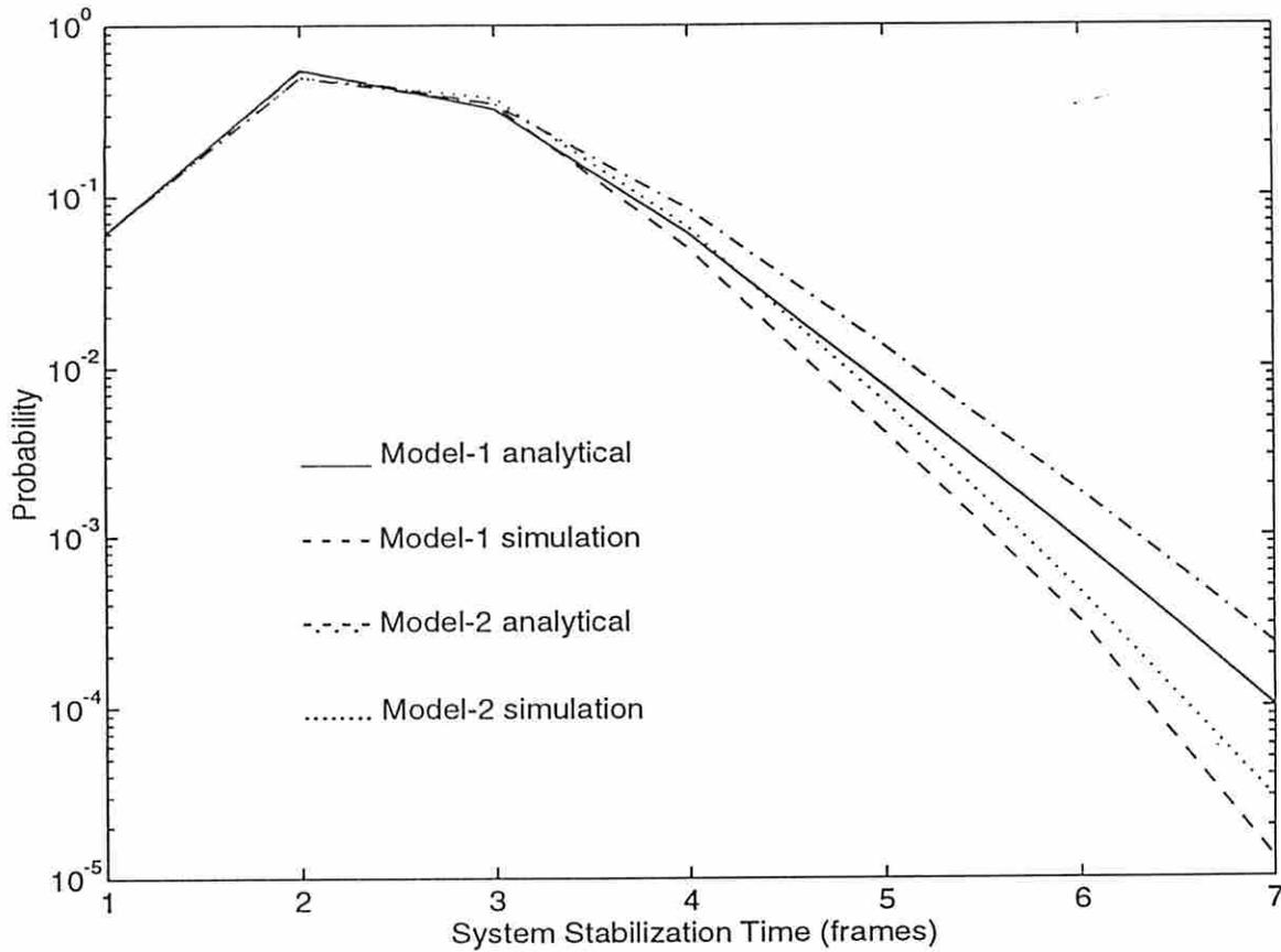
Fig. 4. The probability distribution of the system stabilization time for network A in the worst case. The number of users in the system is 9; the number of slots in a frame is 16.
