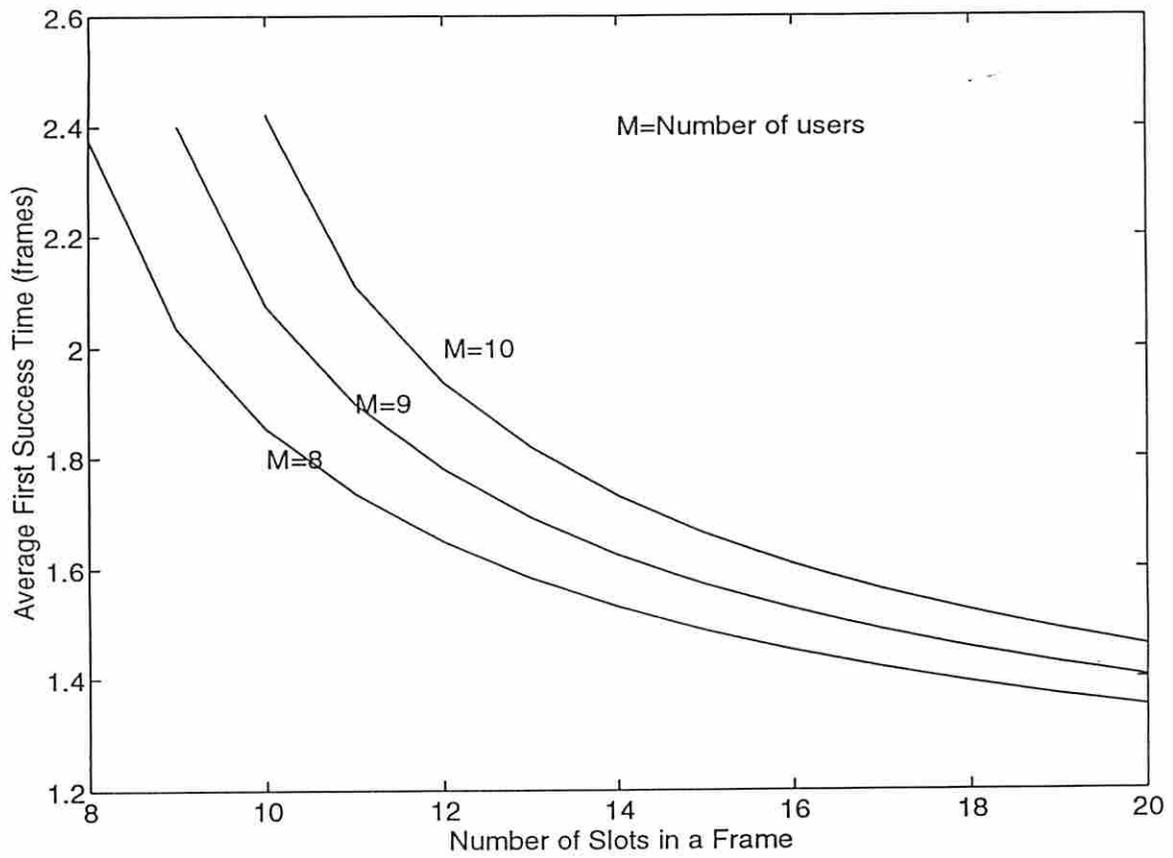
Fig. 7. The average first success time for various values of  $M$  (number of users within an interference range) and  $N$  (number of slots in a frame) for network B in the worst case.
