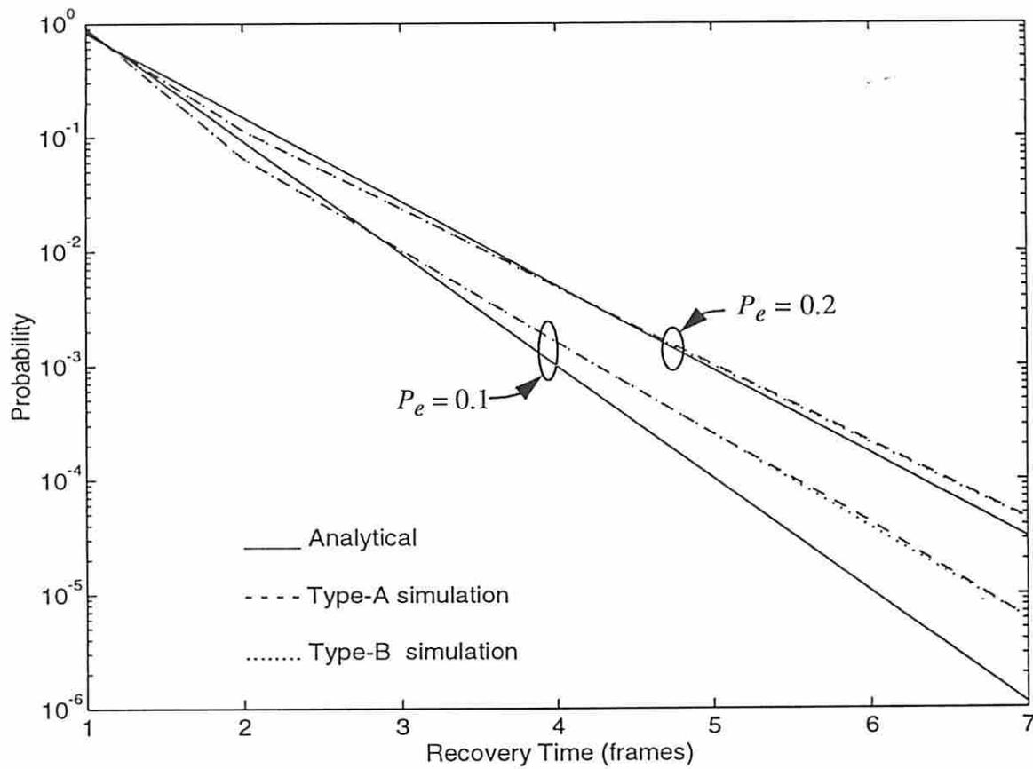
Fig. 8. The probability distribution of the recovery time with the packet error probability  $P_e = 0.1$  and  $0.2$  for networks A and B in the steady state.
