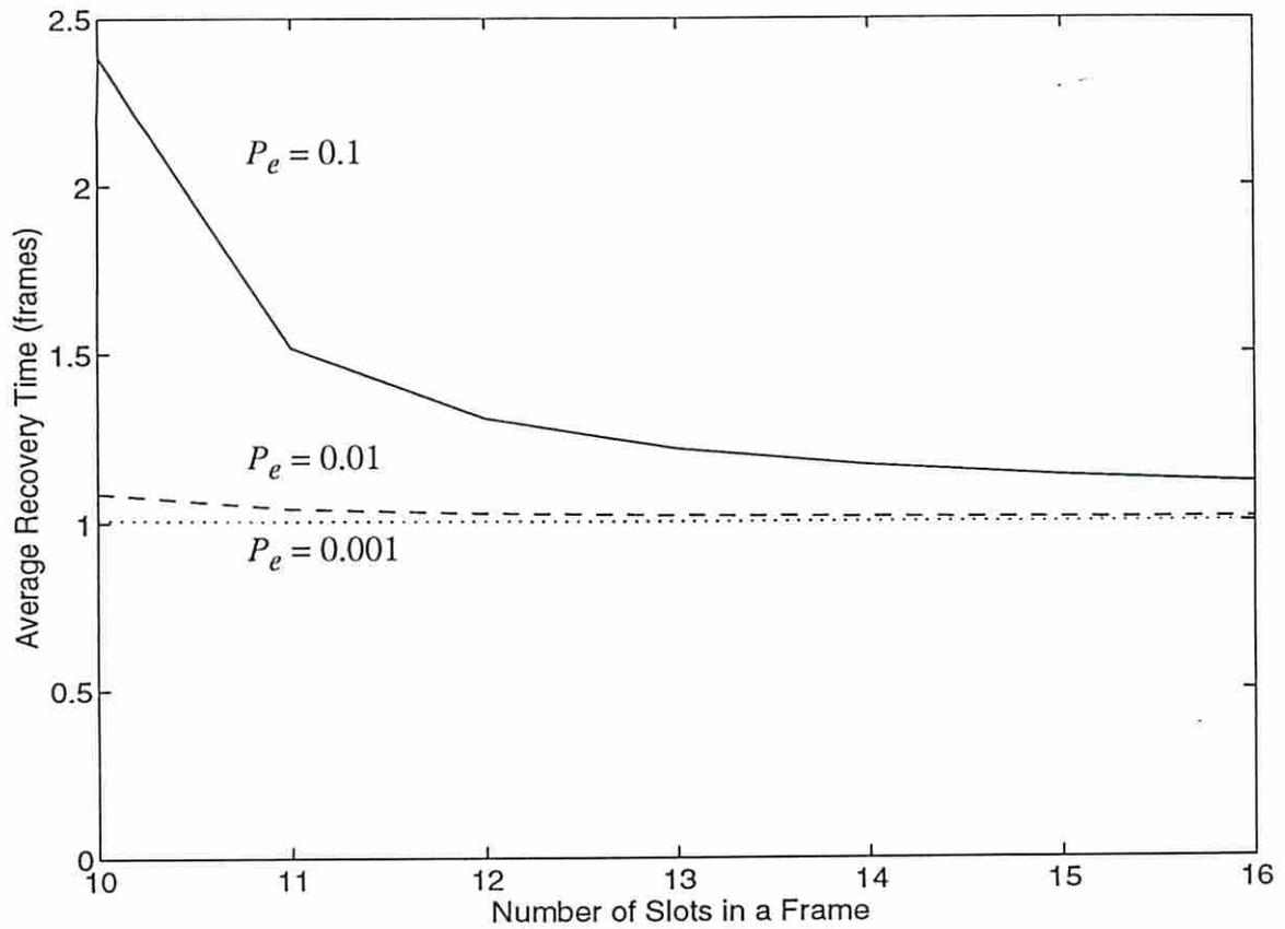
Fig. 9 Average recovery time as a function of the number of slots in a frame and the packet error probability ( $P_e$ ) for network B in the steady state.
