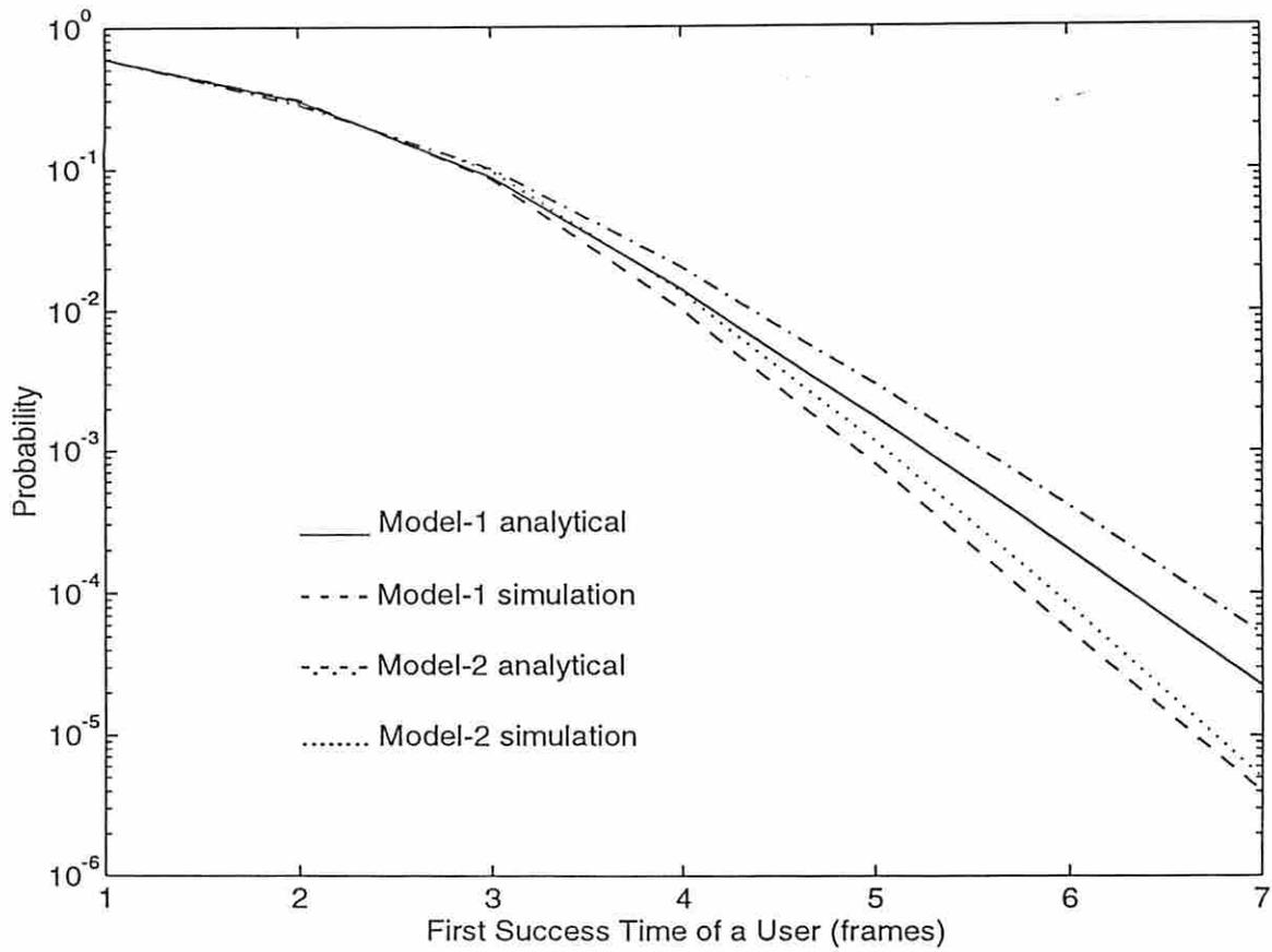
Fig. 6. The probability distribution of the first success time for network B in the worst case. The number of users in the interference range is 9; the number of slots in a frame is 16.
