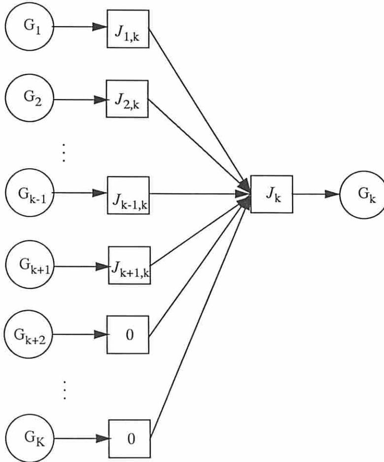
Fig. 3. The flow chart to compute the parameter of the jamming source for group  $k$ .  $J_{i,k}$  is the probability that  $G_i$  jams  $G_k$ .
