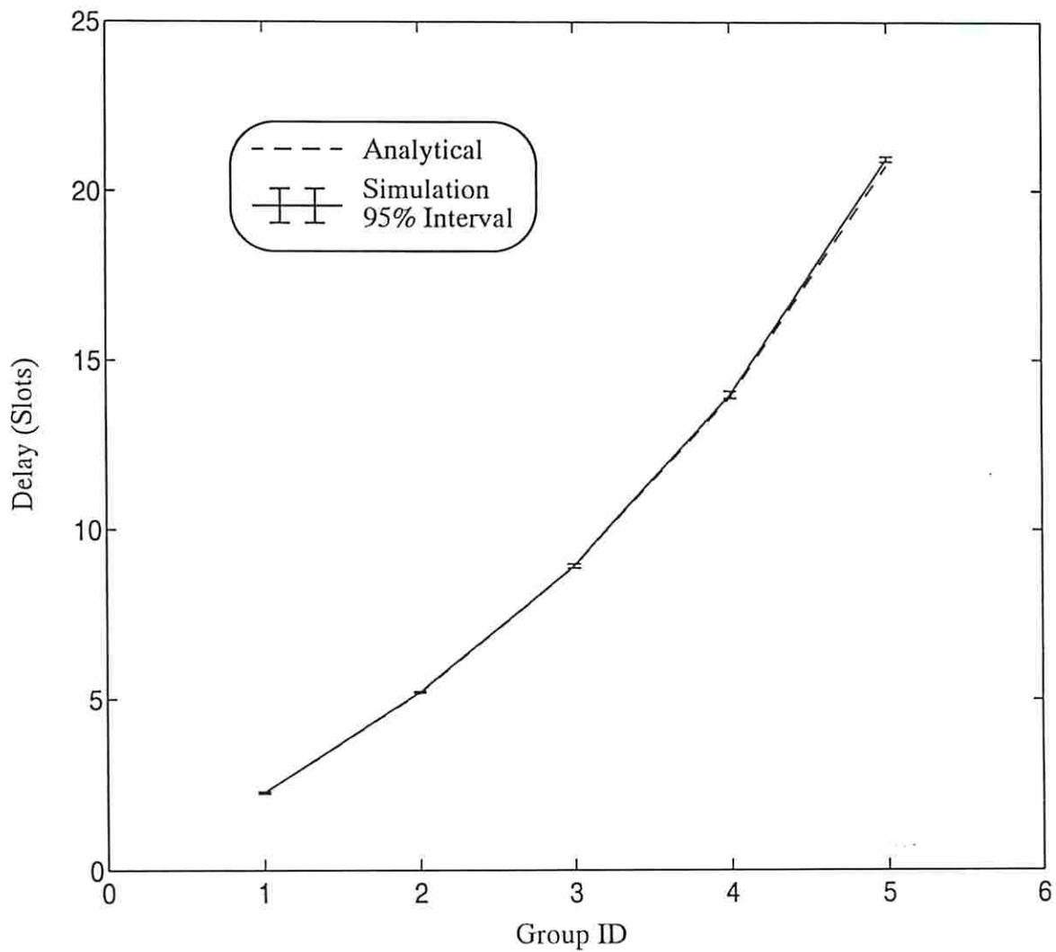
Fig. 5. Delay for a 5-group S-ALOHA system with  $M = 20$ ,  $\sigma = 0.005$ , and  $q = 0.05$  for each group.
