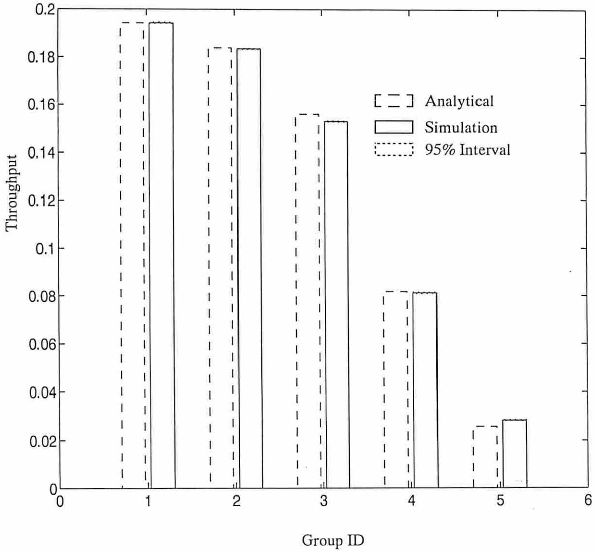
Fig. 8. Throughput for a 5-group S-ALOHA system with  $M = 20$ ,  $\sigma = 0.01$ , and  $q = 0.1$  for each group.
