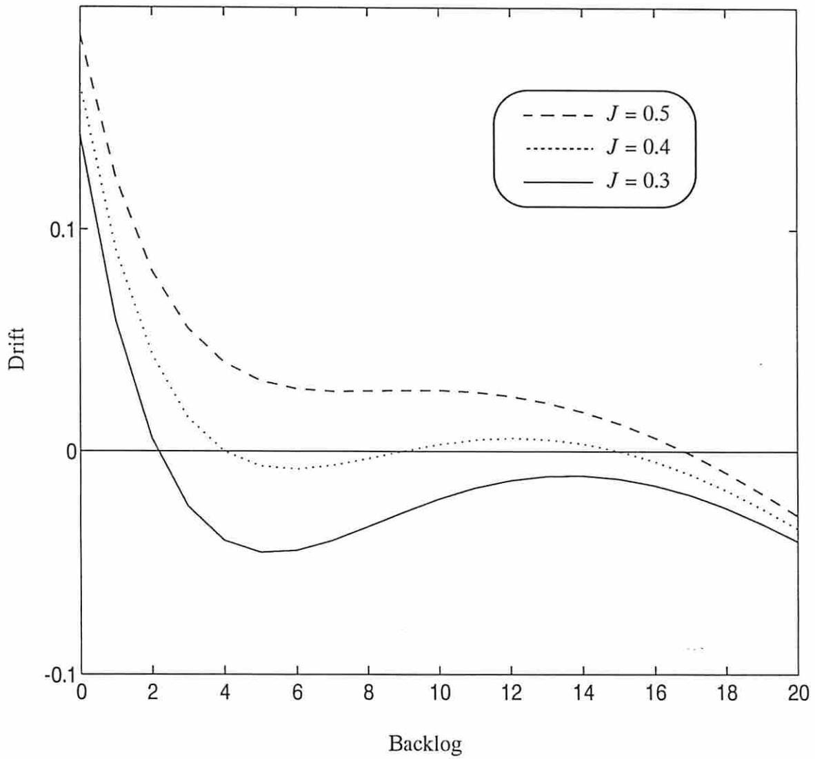
Fig. 2. Drift for S-ALOHA/IBJS with  $M = 20$ ,  $\sigma = 0.015$ , and  $q = 0.2$ .
