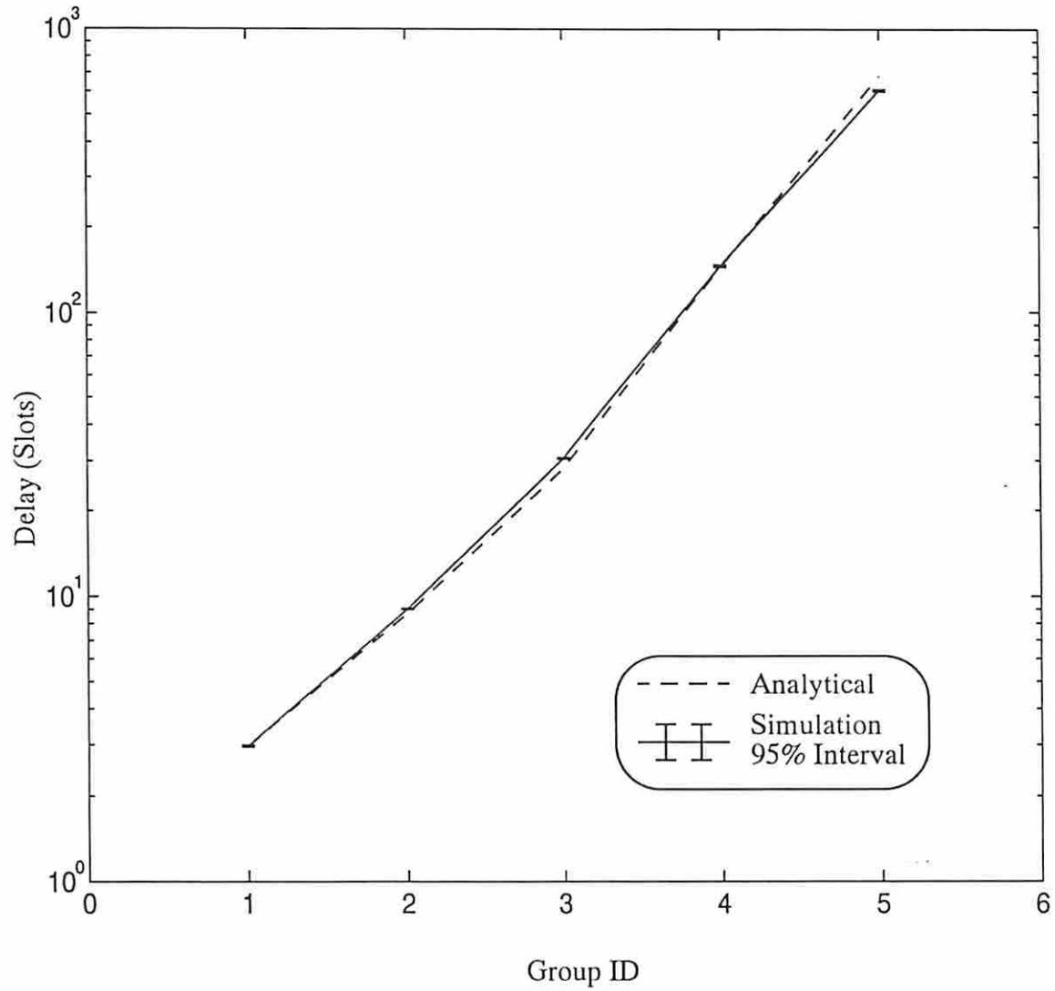
Fig. 9. Delay for a 5-group S-ALOHA system with  $M = 20$ ,  $\sigma = 0.01$ , and  $q = 0.1$  for each group.
