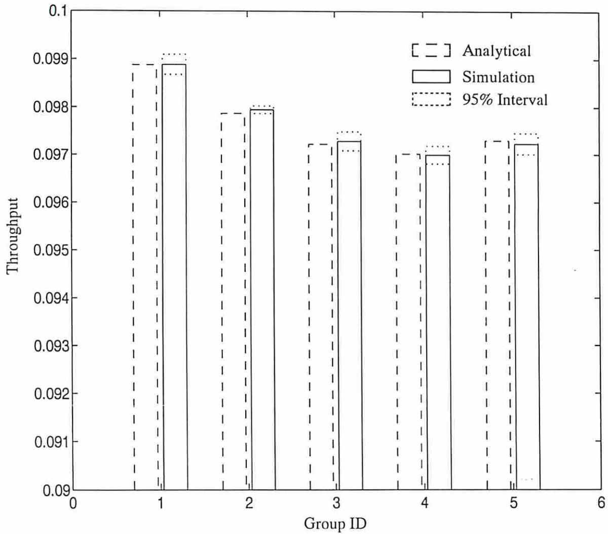
Fig. 6. Throughput for a 5-group S-ALOHA system with parameters for each group as follows:  $G_1$ : ( $M = 20, \sigma = 0.005, q = 0.05$ );  $G_2$ : ( $M = 20, \sigma = 0.005, q = 0.06$ );  $G_3$ : ( $M = 20, \sigma = 0.005, q = 0.08$ );  $G_4$ : ( $M = 20, \sigma = 0.005, q = 0.12$ );  $G_5$ : ( $M = 20, \sigma = 0.005, q = 0.22$ ).
