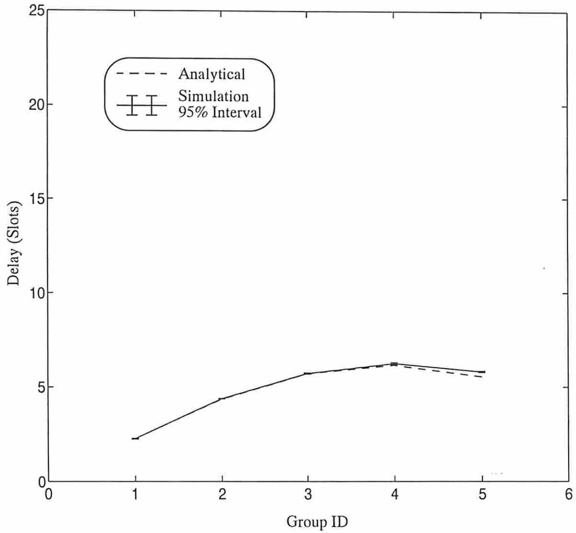
Fig. 7. Delay for a 5-group S-ALOHA system with parameters the same as in Fig. 5.
