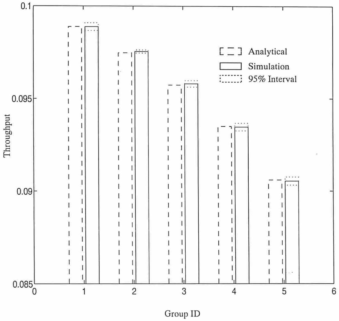
Fig. 4. Throughput for a 5-group S-ALOHA system with  $M = 20$ ,  $\sigma = 0.005$ , and  $q = 0.05$  for each group.
