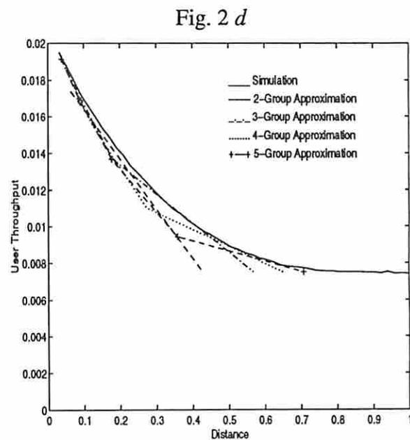
Fig. 2a-2d. The user throughput as a function of the distance relative to the central station for the slotted ALOHA network with Rician fading given in Section 5.1. The transmission probability  $q = 0.02$  and the Rician factor  $K_r = 10$  for all users.
