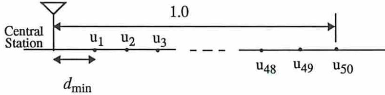
Fig. 1. The topology of a S-ALOHA network with 50 users equally spaced in  $[d_{\min}, 1.0]$ .
