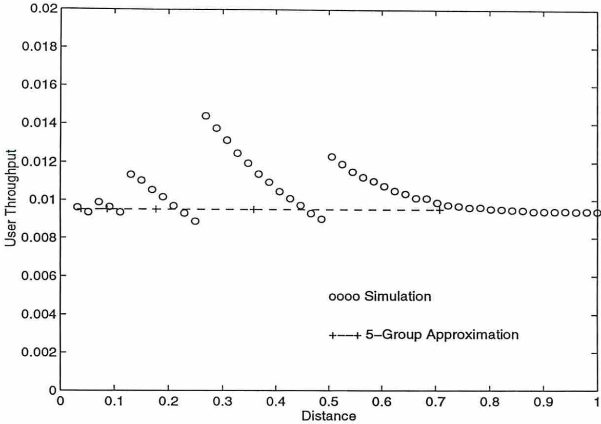
Fig. 3. The user throughput as a function of the distance relative to the central station for the network with Rician fading given in Section 5.1. Users transmit with different probabilities to achieve more balanced throughput, i.e., users 1-2 transmit with probability 0.0097, users 3-5 transmit with probability 0.0105, users 6-12 transmit with probability 0.0132, users 13-24 transmit with probability 0.0222, and users 25-50 transmit with probability 0.0311.
