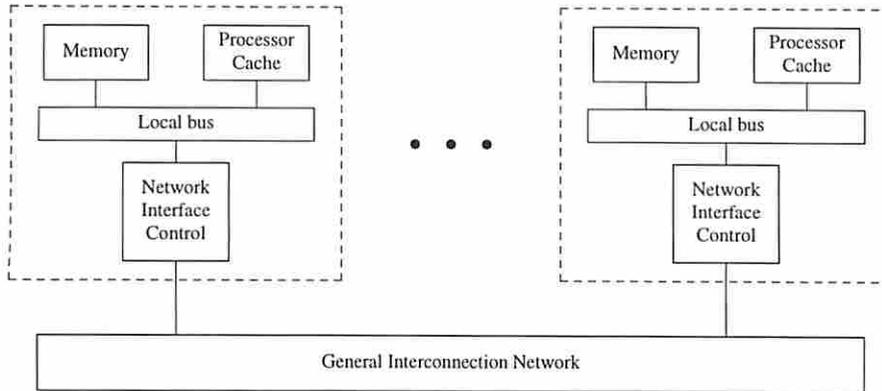
Figure 6: Organisation of a cache coherent multiprocessor.
