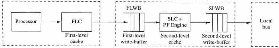
Figure 7: The two-level cache hierarchy in each processing node. The prefetch engine is part of the SLC.
