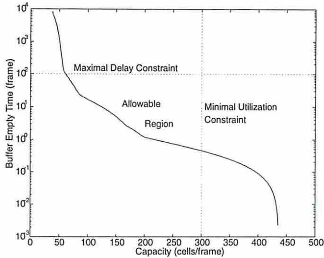
Figure 1: The main fundamental constraints in ATM networks [CG96].
