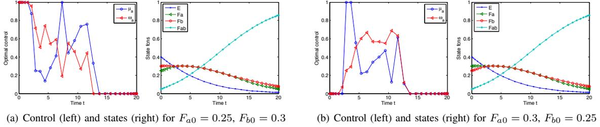
Fig. 2: The two possible structures of the optimal control policy
