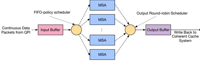
Figure 6. AFU design on FPGA
