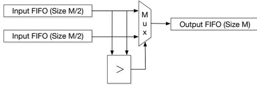
Figure 1. FIFO-based 2-to-1 merge unit
