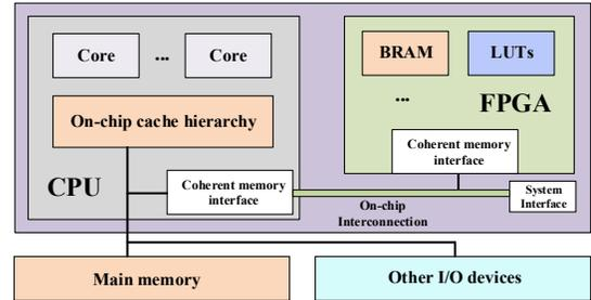
Figure 3. Target architecture integrating general purpose processors and FPGA
