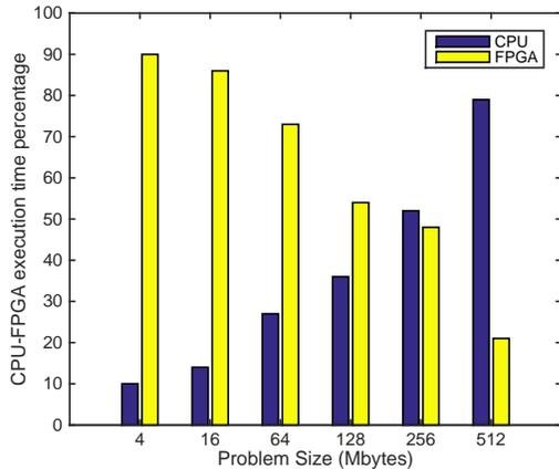
Figure 9. CPU and FPGA execution time break down
