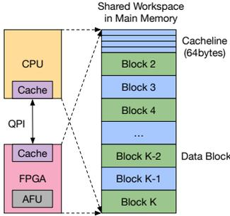
Figure 4. Shared Memory Scheme between CPU and FPGA
