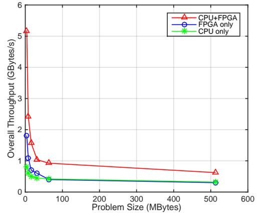
Figure 8. Throughput comparison for various input size
