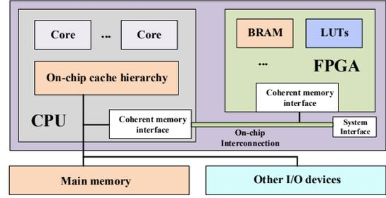
Figure 5: Target architecture integrating general purpose processors and FPGA
