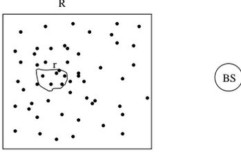
Figure 1: Sensor network to monitor a region R
