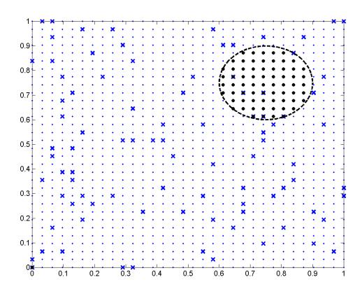
Figure 1: Sample scenario: a distributed sensor network with uncorrelated sensor faults (denoted as 'x') deployed in an environment with a single event region (dashed circle)
