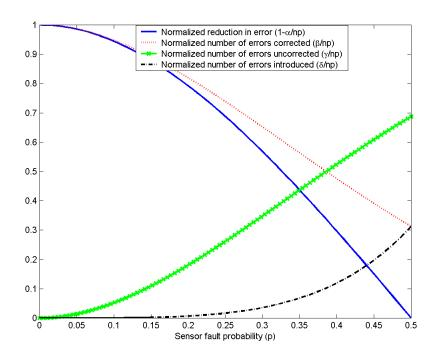
Figure 3: Metrics for the Bayesian fault-recognition algorithm with optimal threshold decision scheme (N=4)
