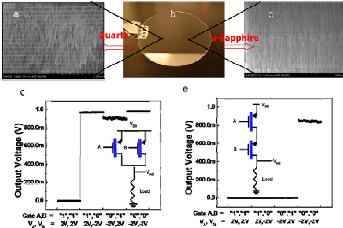
Figure 3: a), c) SEM image of aligned nanotube arrays on quartz and sapphire, respectively. Figure b) photograph of 4 inch substrate with the as-grown nanotubes. Figure d) The NAND logic device data. Inset: schematic diagram of NAND device. Figure e) The NOR logic device data. Inset: schematic diagram of NOR device
