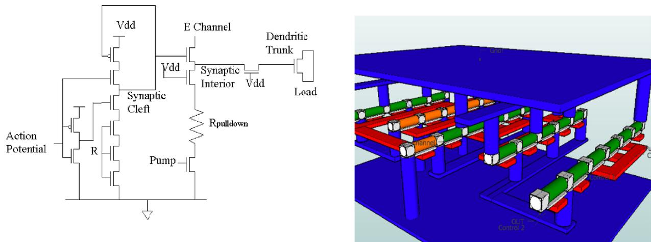
Figure 4: a) The basic synapse circuit used for our volume estimations. b) A 3D model of the basic synapse
